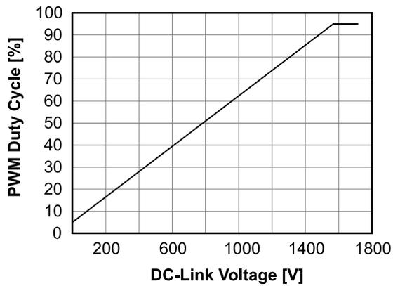
Figure 7. PWM Duty Cycle of DLK vs. Actual DC-Link Voltage (1700 V versions), Conditions:  $T_A = 25\text{ }^\circ\text{C}$ ,  $V_{CC} = 24\text{ V}$
