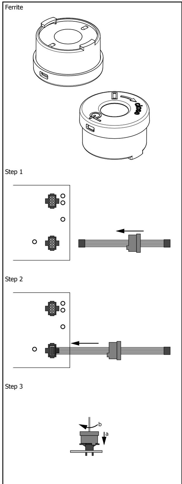
Figure 16. Ferrite Mounting
