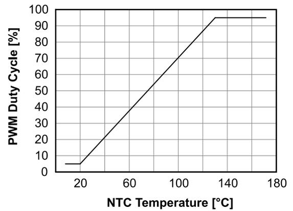
Figure 9. PWM Duty Cycle of Terminal TPM vs. Actual NTC Temperature Measurement
