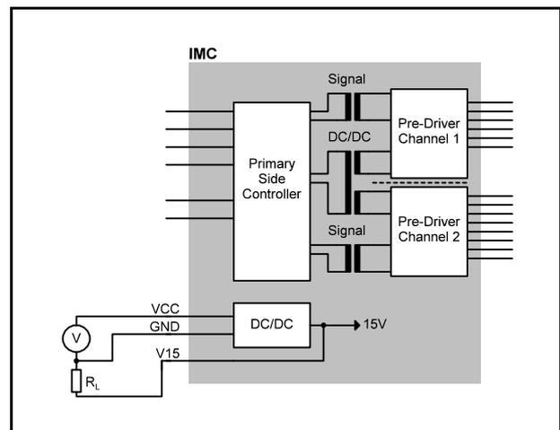
Figure 5. Optional External Load at Terminal V15.
