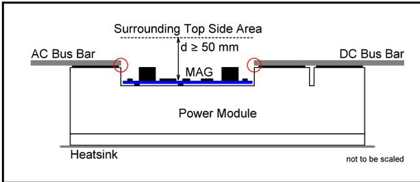
Figure 13. MAG Top Side Clearance Distance to Ensure Proper Cooling.
