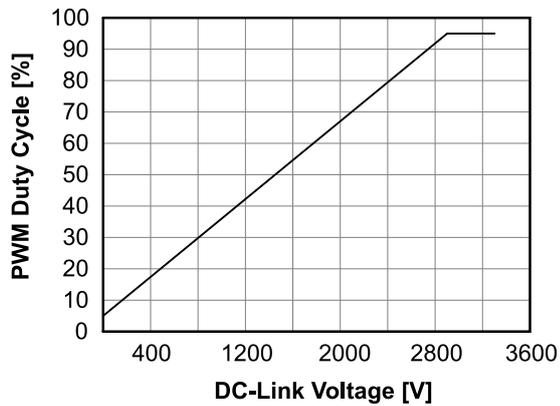
Figure 8. PWM Duty Cycle of DLK vs. Actual DC-Link Voltage (3300 V versions), Conditions:  $T_A = 25\text{ }^\circ\text{C}$ ,  $V_{CC} = 24\text{ V}$
