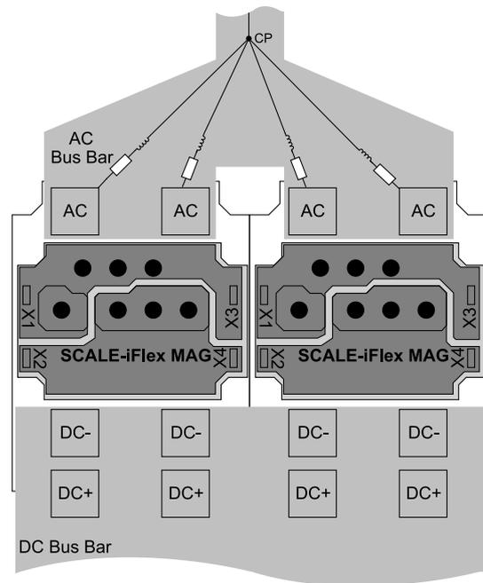
Figure 17. Arrangement of the AC-Busbar for paralleled modules
