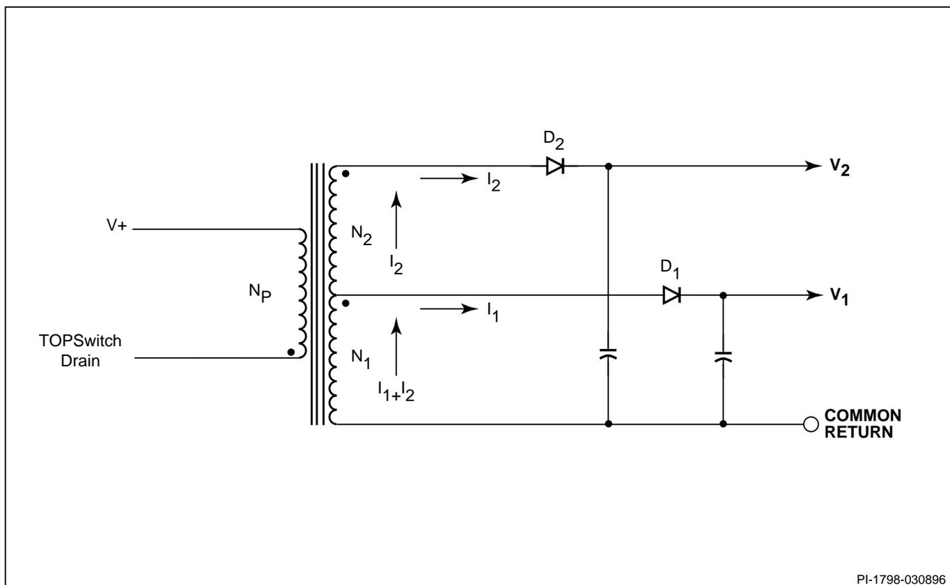
Figure 8. Stacked Secondary Windings for Multiple Outputs.
