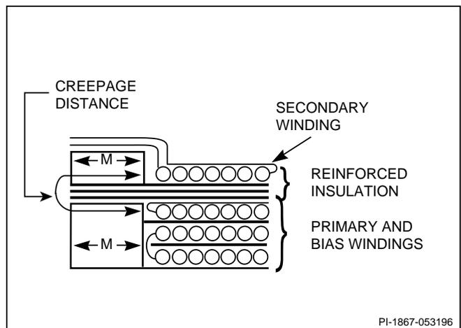
Figure 3. Interwinding Creepage Distance for Margin Wound Transformers.
