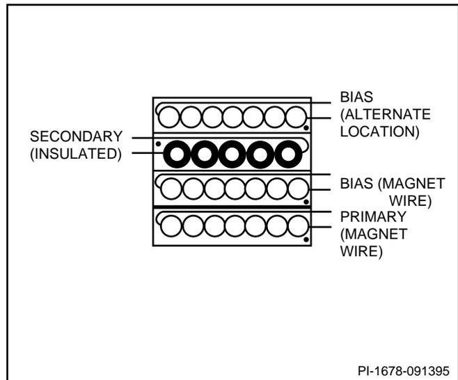
Figure 6. Triple Insulated Wire Wound Transformer Cross Section.
