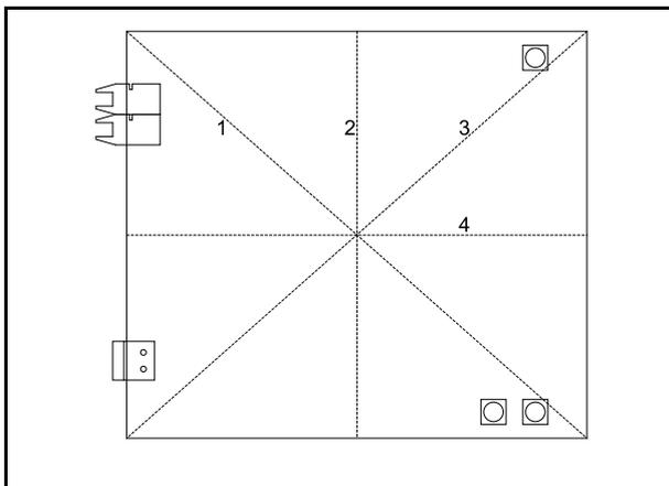
Figure 8. Bending Lines
