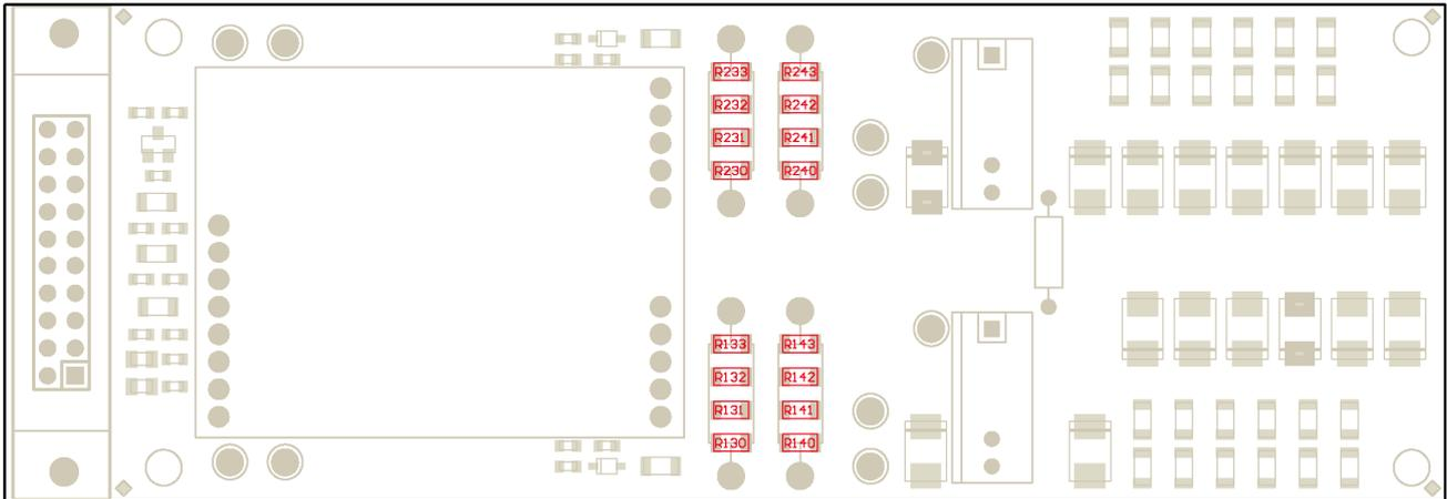
Fig. 4: Assembly drawing of 2BB0108T with highlighted SMD gate resistors
