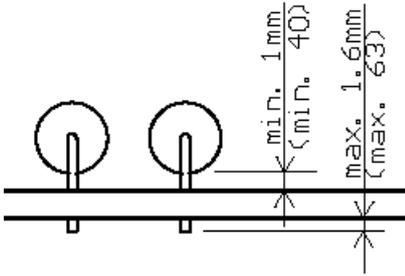
Fig. 6: Minimum and maximum distances when soldering THT gate resistors (in mm/mil)
