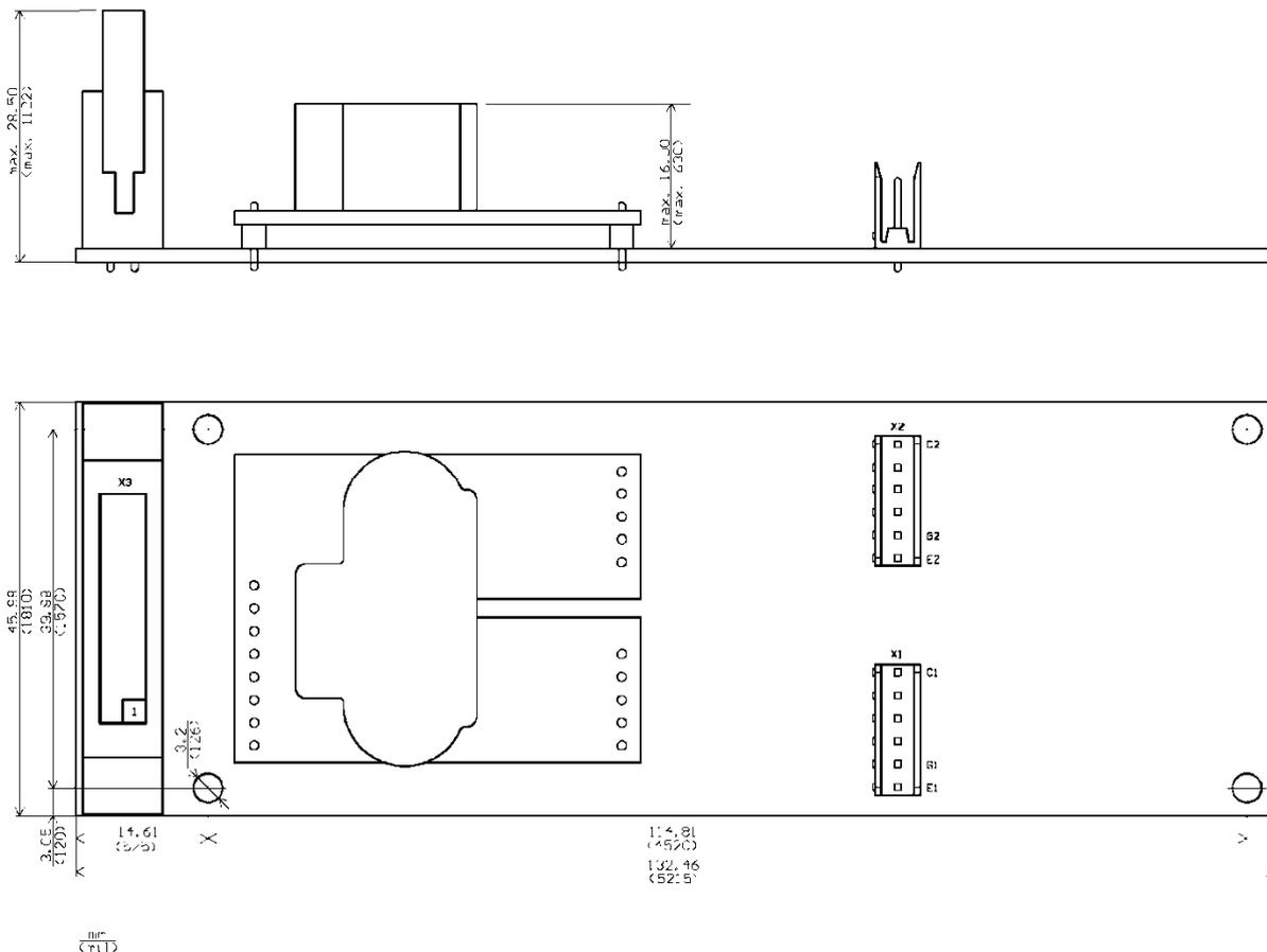
Electrical connector on the Base Board: 71918-120LF from FCI
