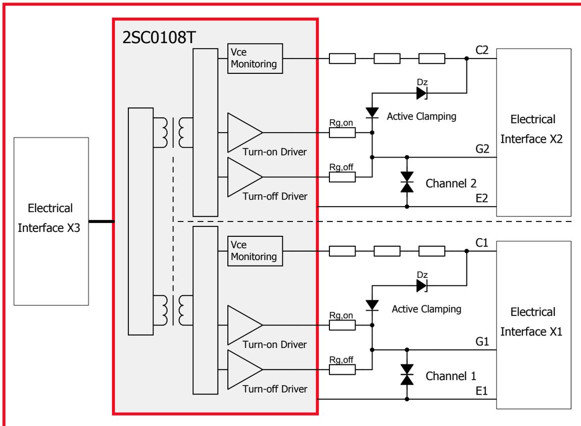
Fig. 2 Basic schematic of the 2BB0108T Base Board with 2SC0108T driver
