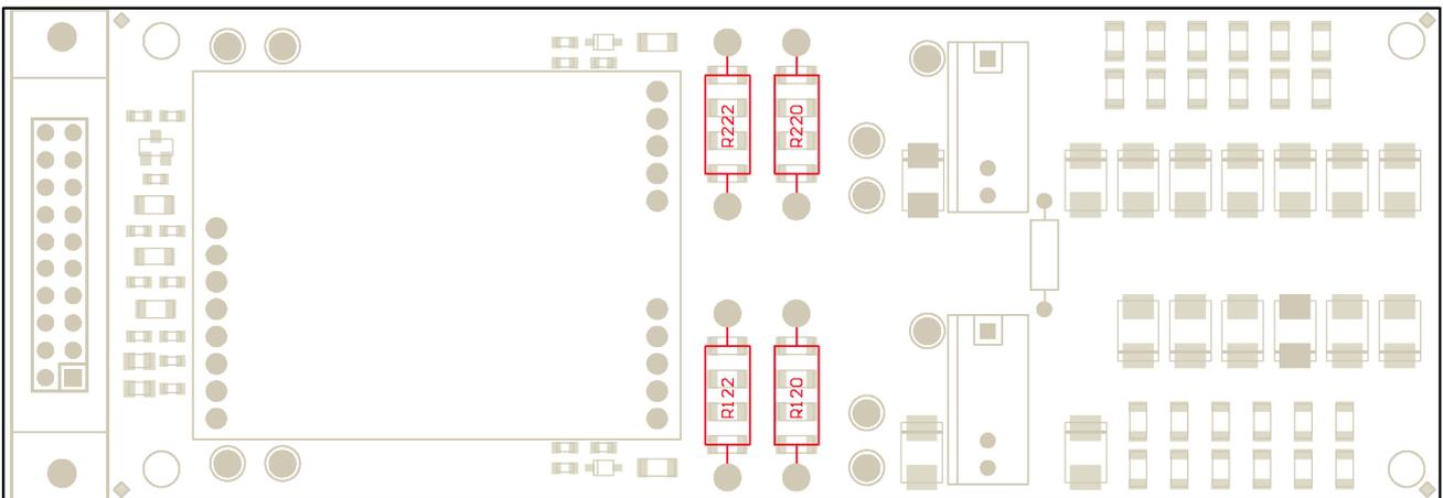
Fig. 5: Assembly drawing of 2BB0108T with highlighted THT gate resistors
