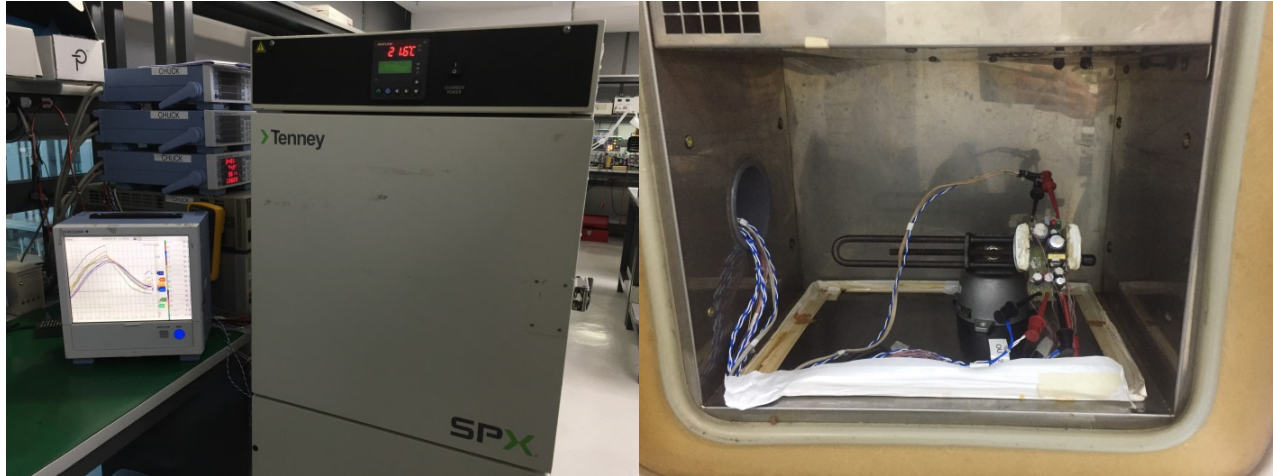
Figure 147 – Thermal Performance Set-up using Thermal Chamber.
