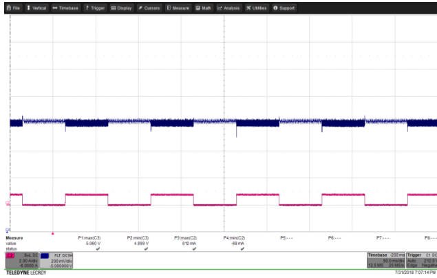
Figure 56 – Transient Response. 85 VAC, 5.0 V, 0 – 0.75 A Load Step. V_{MIN} : 4.899 V, V_{MAX} : 5.060 V. Upper: V_{OUT} , 0.2 V / div., 50 ms / div. Lower: I_{LOAD} , 2 A / div.
