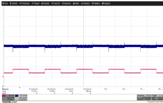
Figure 74 – Transient Response. 85 VAC, 15.0 V, 0.75 – 1.5 A Load Step. V_{MIN} : 14.885 V, V_{MAX} : 15.102 V. Upper: V_{OUT} , 0.2 V / div., 50 ms / div. Lower: I_{LOAD} , 2 A / div.
