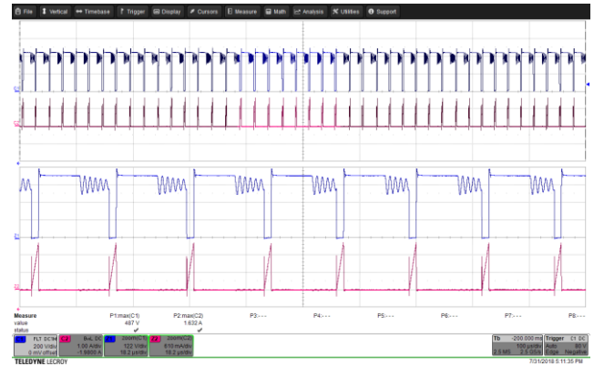
Figure 91 – Drain Voltage and Current Waveforms. 265 VAC, 9 V, 3 A Load (487.0 V_{MAX} ). Upper: V_{DRAIN} , 200 V, 100 \mu s / div. Lower: I_{DRAIN} , 1 A / div.
