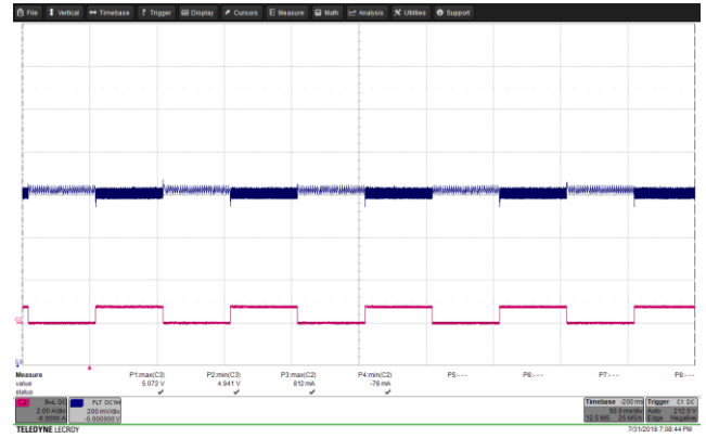
Figure 57 – Transient Response. 265 VAC, 5.0 V, 0 – 0.75 A Load Step. V_{MIN} : 4.941 V, V_{MAX} : 5.072 V. Upper: V_{OUT} , 0.2 V / div., 50 ms / div. Lower: I_{LOAD} , 2 A / div.
