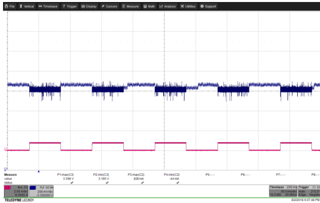
Figure 48 – Transient Response. 85 VAC, 3.3 V, 0 – 0.75 A Load Step. V_{MIN} : 3.195 V, V_{MAX} : 3.398 V. Upper: V_{OUT} , 0.2 V / div., 50 ms / div. Lower: I_{LOAD} , 2 A / div.
