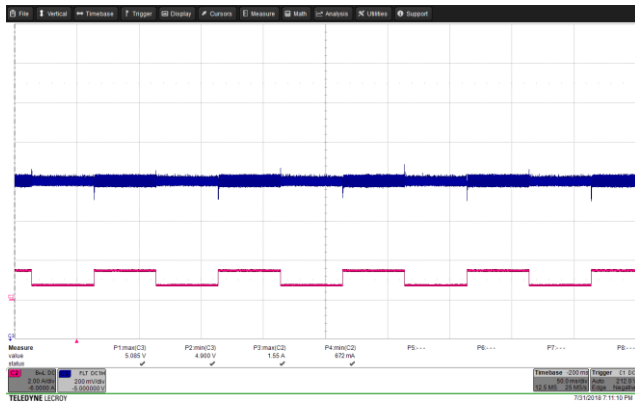
Figure 58 – Transient Response. 85 VAC, 5.0 V, 0.75 – 1.5 A Load Step. V_{MIN} : 4.900 V, V_{MAX} : 5.085 V. Upper: V_{OUT} , 0.2 V / div., 50 ms / div. Lower: I_{LOAD} , 2 A / div.
