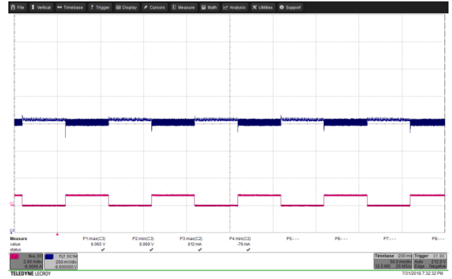
Figure 65 – Transient Response. 265 VAC, 9.0 V, 0 – 0.75 A Load Step. V_{MIN} : 8.899 V, V_{MAX} : 9.065 V. Upper: V_{OUT} , 0.2 V / div., 50 ms / div. Lower: I_{LOAD} , 2 A / div.
