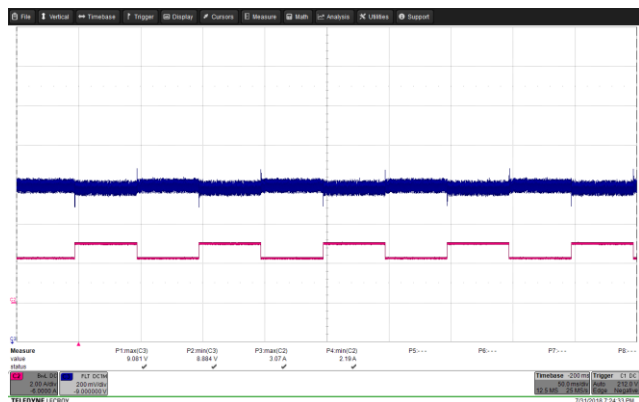
Figure 70 – Transient Response. 85 VAC, 9.0V, 2.25 – 3 A Load Step. V_{MIN} : 8.884 V, V_{MAX} : 9.081 V. Upper: V_{OUT} , .2 V / div., 50 ms / div. Lower: I_{LOAD} , 2 A / div.
