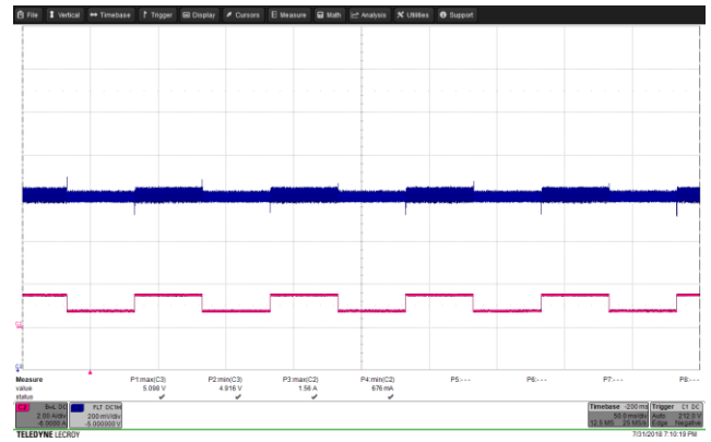
Figure 59 – Transient Response. 265 VAC, 5.0 V, 0.75 – 1.5 A Load Step. V_{MIN} : 4.961 V, V_{MAX} : 5.098 V. Upper: V_{OUT} , 0.2 V / div., 50 ms / div. Lower: I_{LOAD} , 2 A / div.
