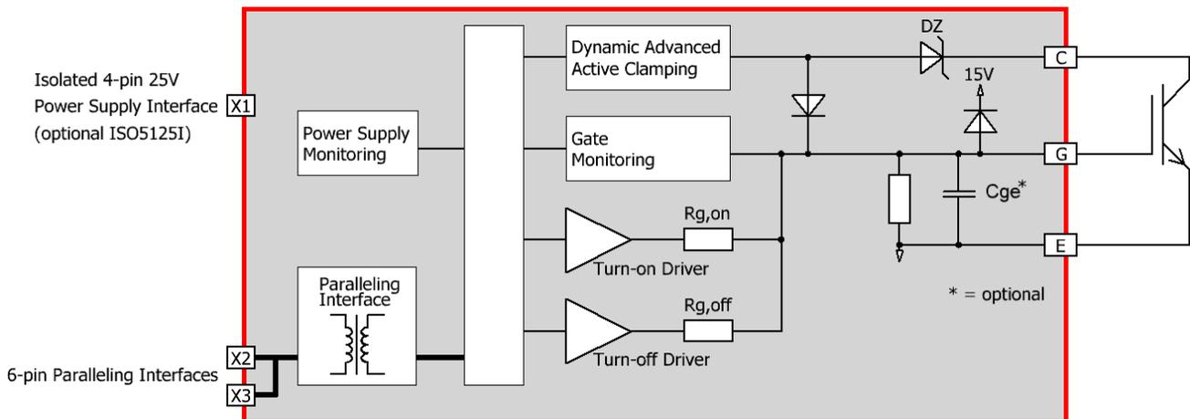
Fig. 3 Basic schematic of the 1SP0335D drivers
