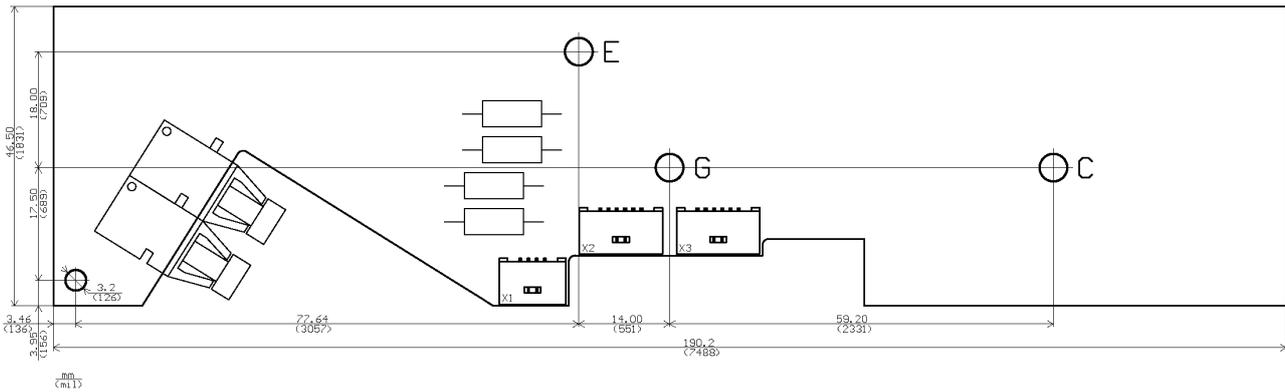
Maximum driver height: 10mm measured from the bottom layer
