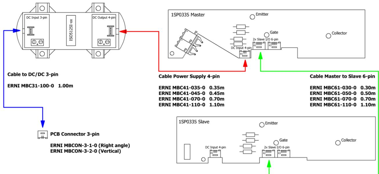
Fig. 11 Cable arrangement for 1SP0335 (Master only or Master and Slave) and DC-DC converter ISO5125I
