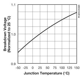
Figure 16. Breakdown vs. Temperature.
