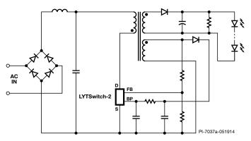
Figure 1. Typical Flyback Implementation – Not a Simplified Circuit.
