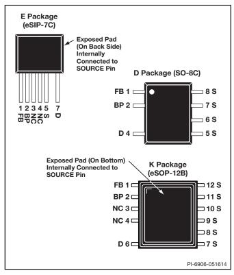
Figure 3. Pin Configuration.
