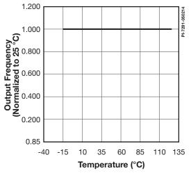
Figure 11. Output Frequency vs. Temperature.
