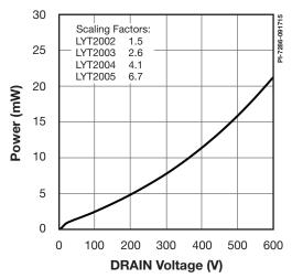
Figure 19. Drain Capacitance Power.
