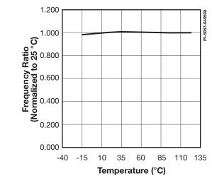
Figure 12. Frequency Ratio vs. Temperature (Constant Current).
