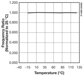
Figure 13. Frequency Ratio vs. Temperature (Inductor Current).
