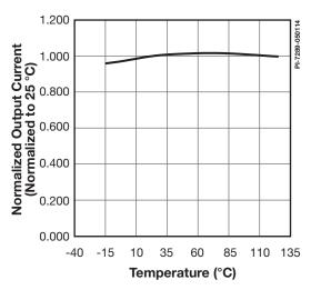
Figure 15. Normalized Output Current vs. Temperature.
