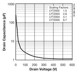
Figure 18.  $C_{\rm OSS}$  vs. Drain Voltage.
