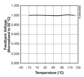
Figure 14. Feedback Voltage vs. Temperature.
