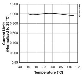
Figure 10. Current Limit vs. Temperature.
