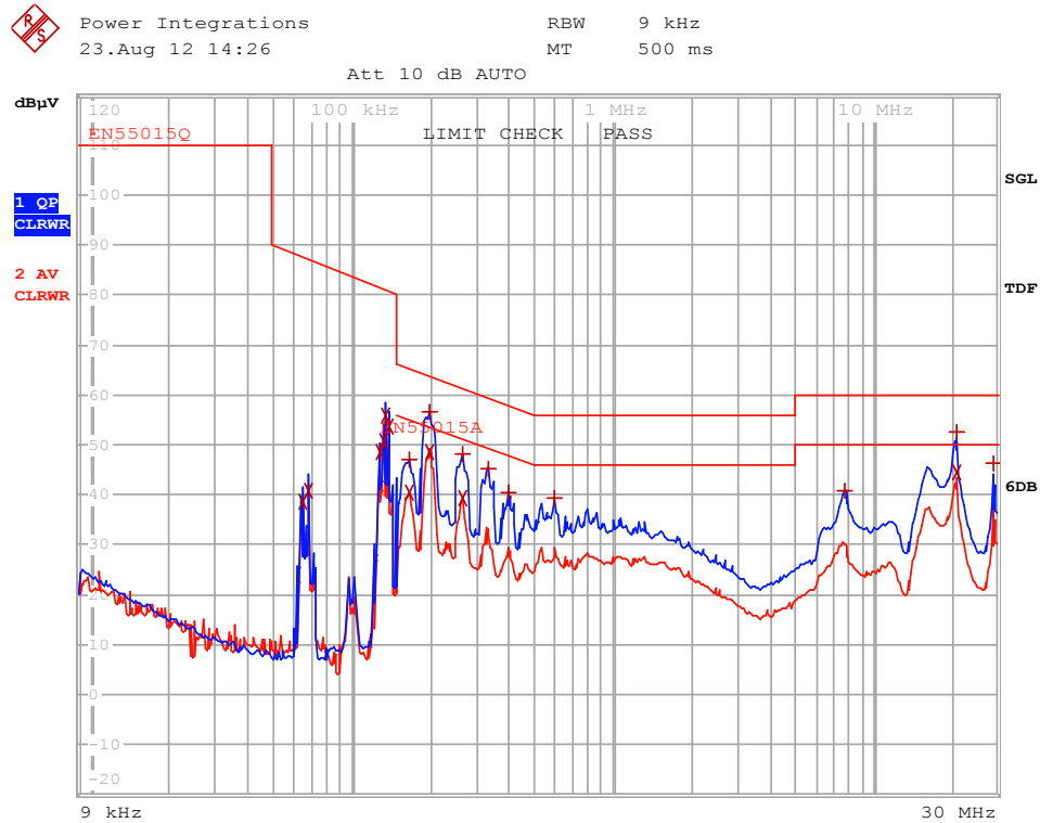
Figure 33 – 30 V LED Load, 230 VAC, 60 Hz, and EN55015 Limits.
