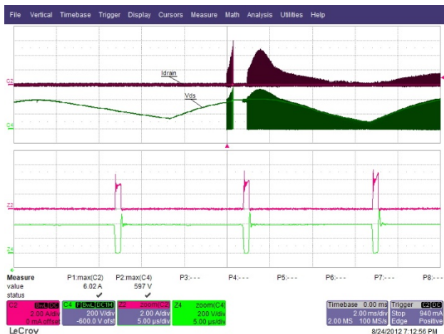
Figure 22 – 277 VAC 50 Hz., Full Load Start-up. Upper: I_{DRAIN} , 2 A / div. Lower: V_{DRAIN} , 200 V, 2 ms / div.
