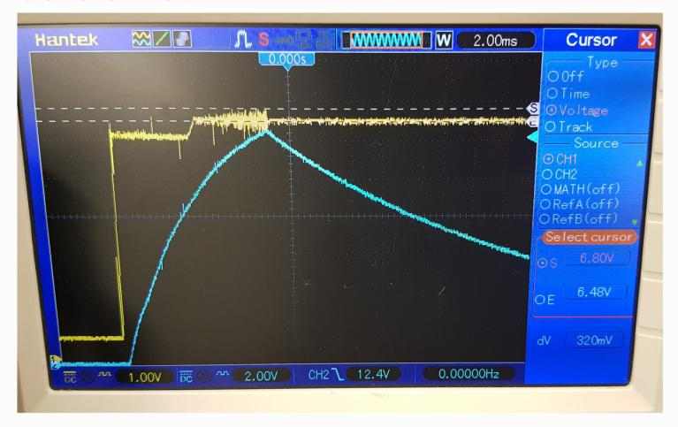
V(BP, S) = 6.1V after boot, and increases to about 6.5V after 6ms. Then signal gets a bit noisy and when shutdown the voltage settles down at 6.5V.
