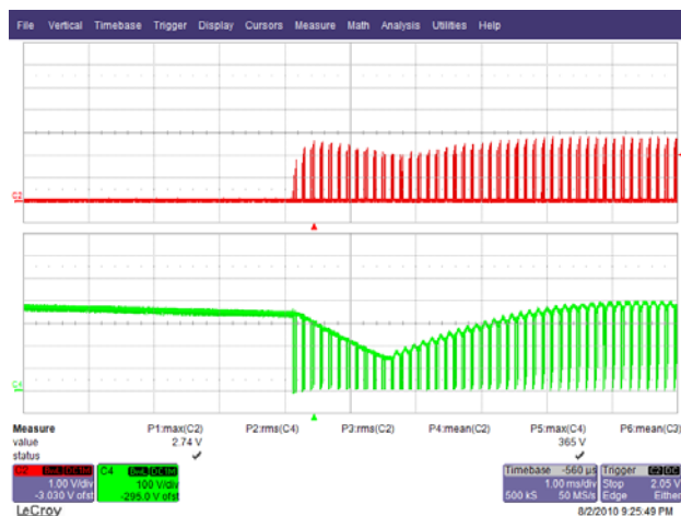
Figure 41 – 265 VAC 60 Hz, Output Short. Upper: I_{DRAIN} , 1 A / div. Lower: V_{DRAIN} , 100 V, 10 ms / div.
