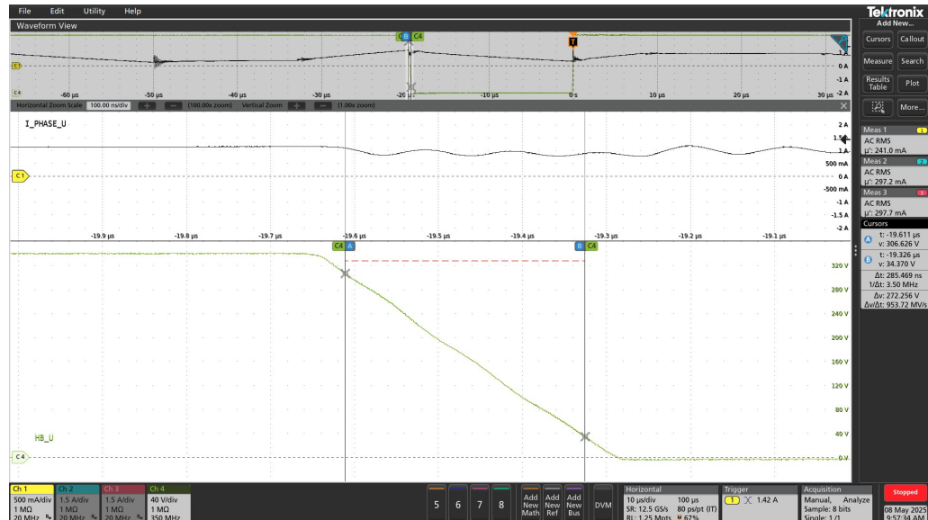
Figure 17 – Low-side V_{DS} Turn-On Slew Rate of Phase U at Light Load (Positive Peak).
