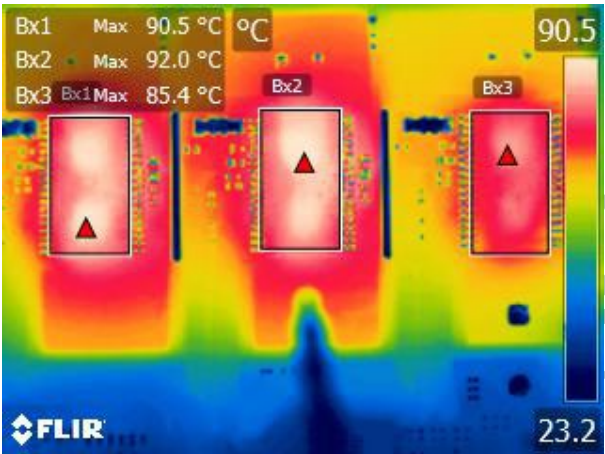
Figure 42 – Thermal Scan at 2.26 ARMS Ambient = 23.5 °C.
