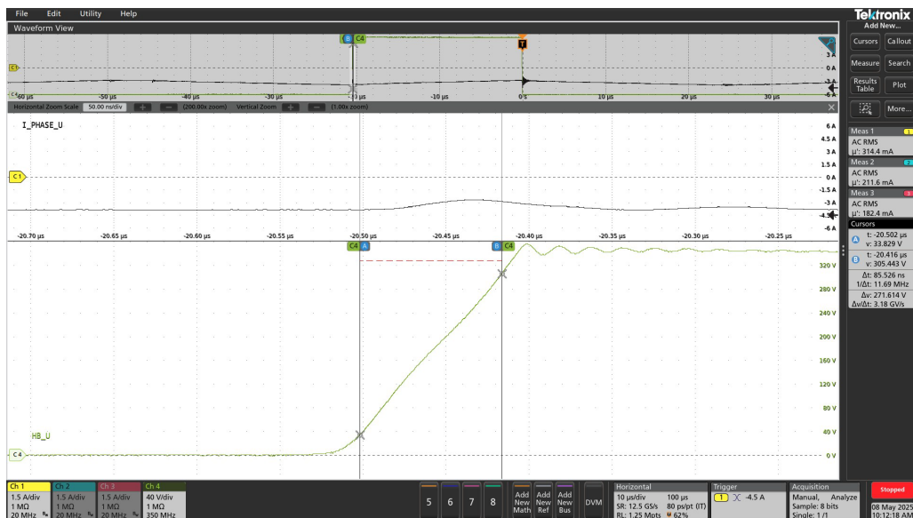
Figure 24 – Low-side V_{DS} Turn-Off Slew Rate of Phase U at Full Load (Negative Peak).
