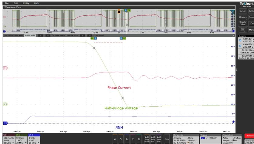
**Figure 27** – Drain Voltage (Turn-On) 70 W Inverter Output Power.
