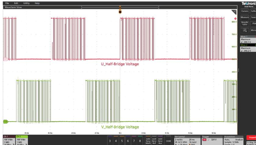
**Figure 18** – Half-Bridge Voltages at 35 W Inverter Output Power.
