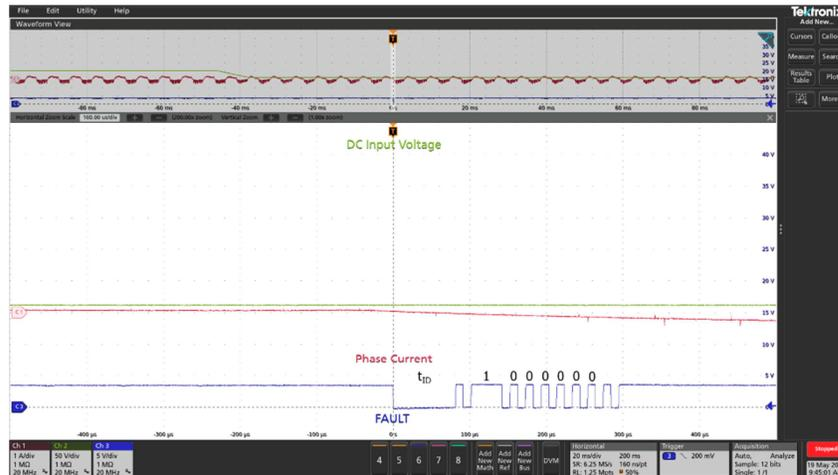
**Figure 34** – 200 to 160  $V_{DC}$ , Slew Rate: 5 V / ms.
