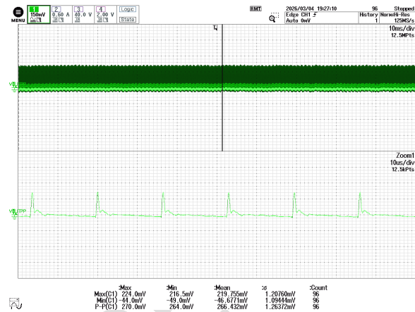
Figure 86 – Output Voltage Ripple. 100 VDC, 1 A, 25 °C Ambient CH1: V_{OUT} , 150 mV / div. Time: 10 ms / div.
