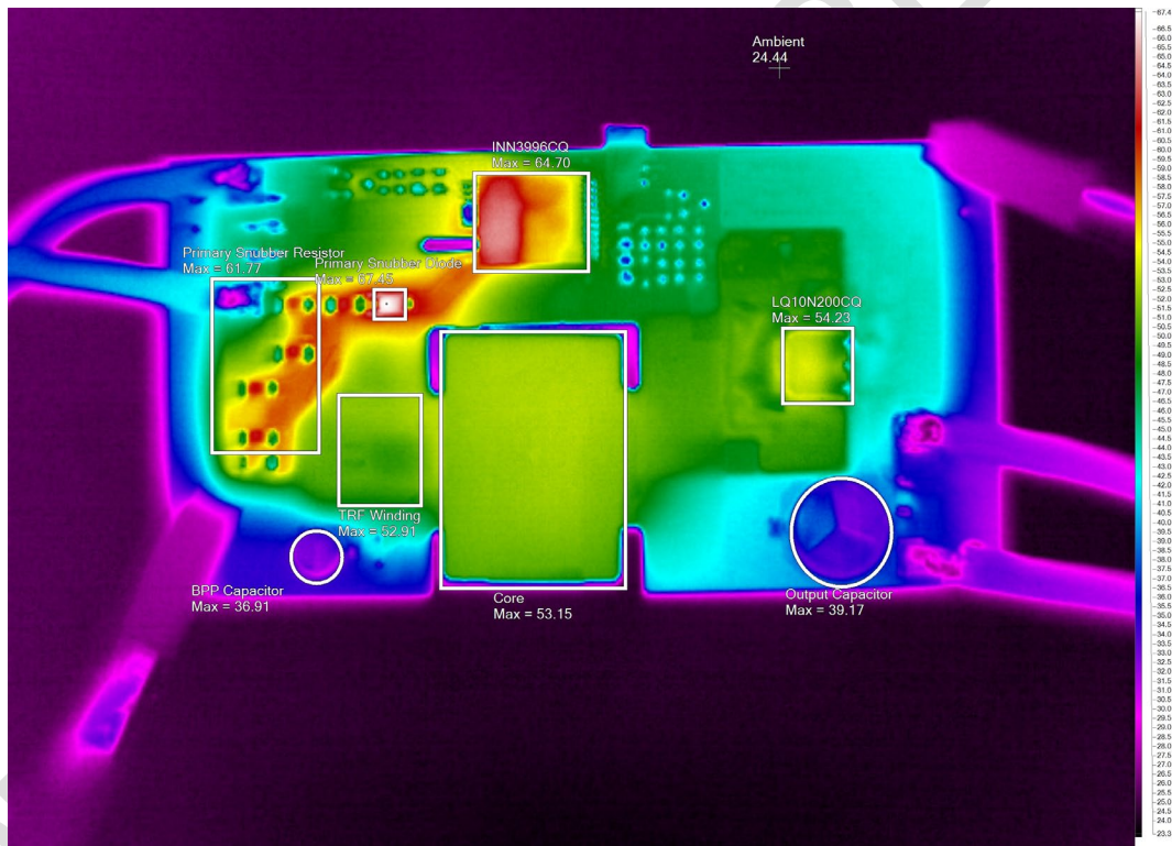
Figure 24 – Thermal Scan at 500 VDC Input, 1 A Load.
