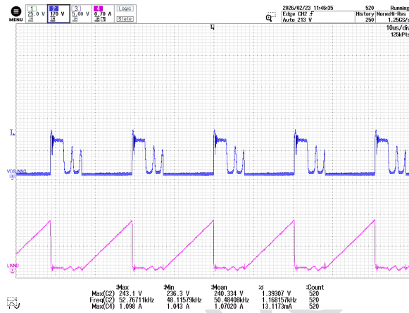
Figure 52 – INN3996CQ Drain Voltage and Current. 40 VDC, 0.67A Load. CH2: V_{DS,INNO} , 170 V / div. CH4: I_{DS,INNO} , 700 mA / div. Time: 10 \mu s / div
