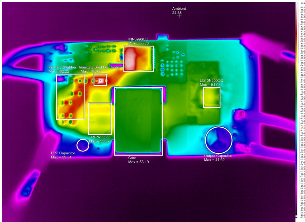
Figure 25 – Thermal Scan at 100 VDC Input, 1 A Load.
