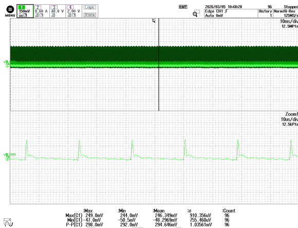
Figure 87 – Output Voltage Ripple. 400 VDC, 0.67 A, 25 °C Ambient CH1: V_{OUT} , 150 mV / div. Time: 10 ms / div.
