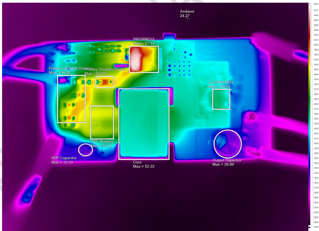
Figure 26 – Thermal Scan at 40 VDC Input, 0.67 A Load.
