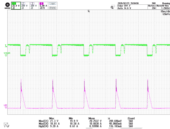
Figure 60 – Q-Speed Diode Voltage and Current. 40 VDC, 0.67A Load. CH1: V_{KA,QSP} , 25 V / div. CH4: I_{DS,INNO} , 5 A / div. Time: 10 \mu s / div
