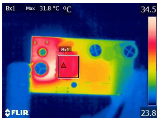
Figure 97 – 265 VAC 50 Hz. Output Short, Top. 1 Hour Soak Ambient = 23.8 °C Transformer = 31.8 °C
