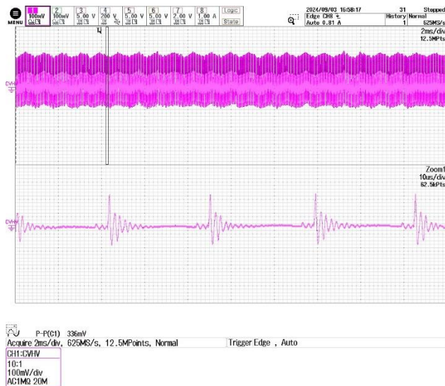
(g) 800 VDC Input Line Voltage V_{\text{RIPPLE\_CVHV}} = 336 \text{ mV}
