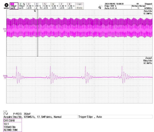
(h) 1000 VDC Input Line Voltage V_{\text{RIPPLE\_CVHV}} = 352 \text{ mV}
