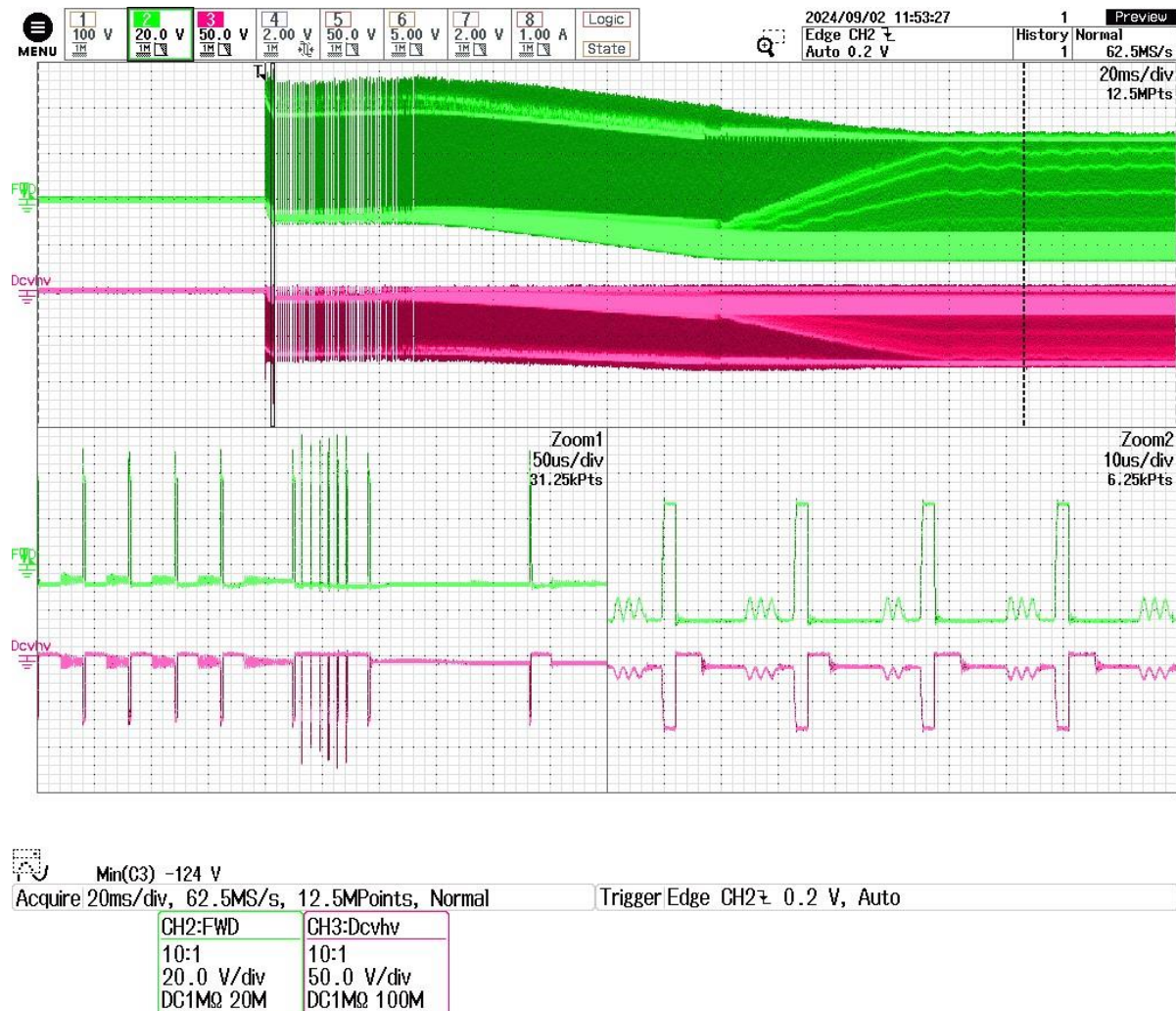
Figure 21 – CVHV Diode Worst Case Reverse Voltage, V_{D3\_PK} = 124\text{ V}
