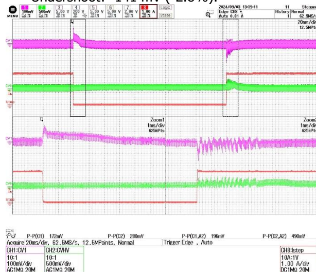
(b) 1000 VDC, ICV1 = 0 A -> 2.5 A (100%) -> 0 A. ICVHV = 0 A. Overshoot: 140 mV (2.8%). Undershoot: -141 mV (-2.8%).
