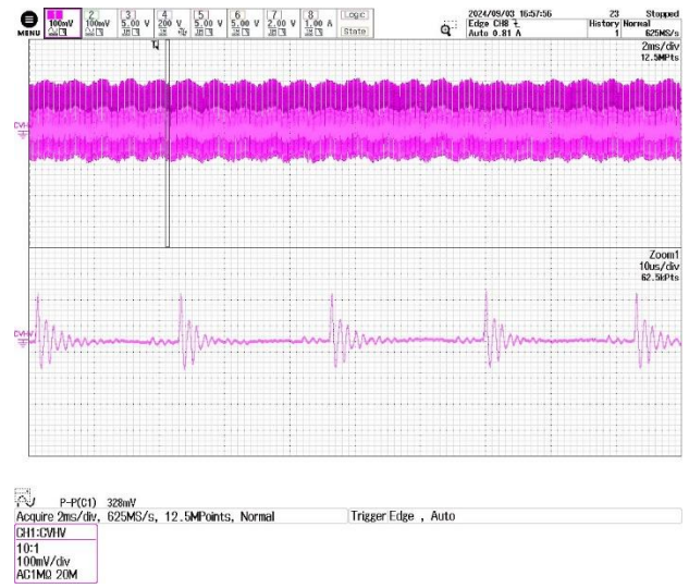
(f) 500 VDC Input Line Voltage V_{\text{RIPPLE\_CVHV}} = 328 \text{ mV}
