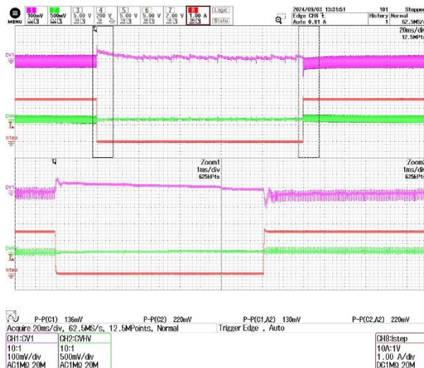
(a) 300 VDC, ICV1 = 0 A -> 2.5 A (100%) -> 0 A. ICVHV = 0 A. Overshoot: 136 mV (2.7%). Undershoot: -130 mV (-2.6%).
