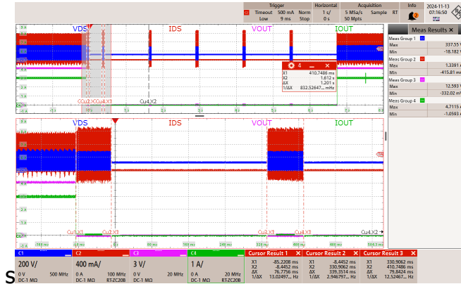
Figure 93 – 85 VAC 60 Hz. Output Short.
