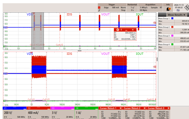
Figure 91 – 85 VAC 60 Hz. Output Short.
