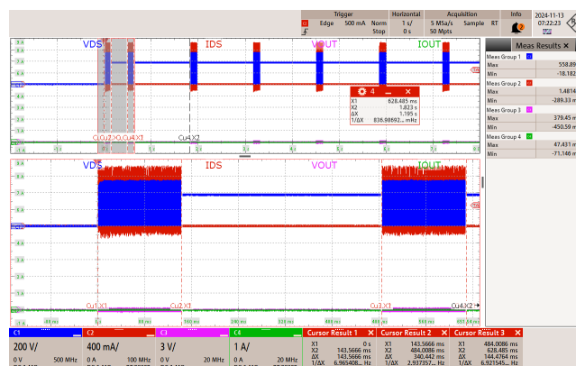
Figure 92 – 265 VAC 50 Hz Output Short.
