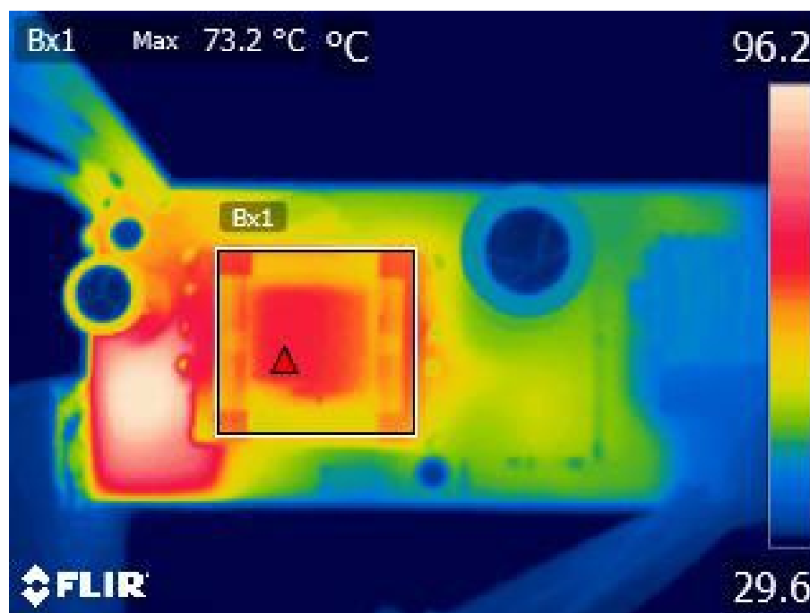
Figure 89 – 265 VAC 50 Hz. Top Side Discrete Component Thermals.
