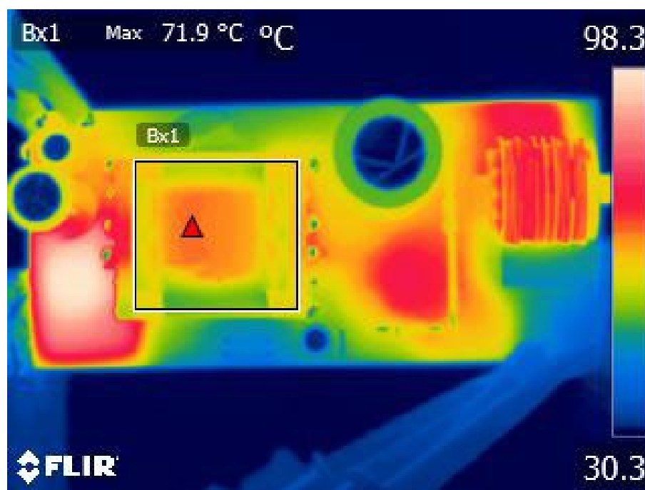
Figure 87 – 85 VAC 60 Hz. Top Side Discrete Component Thermals.
