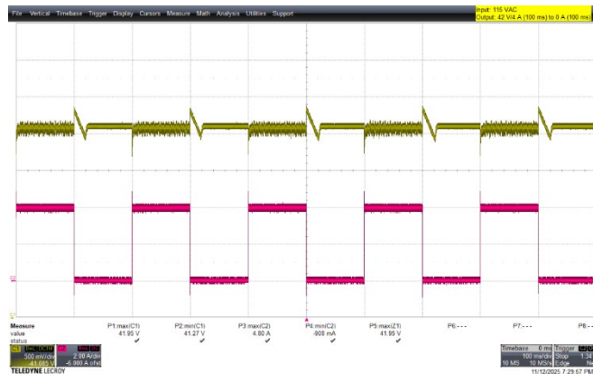
Figure 19 – 115 VAC, 60 Hz. I_o = 0 - 4 A (0-100%) load step.
