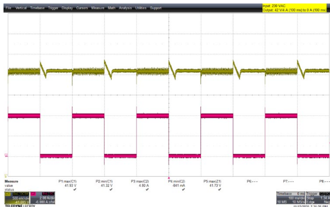
Figure 20 – 230 VAC, 50 Hz. I_o = 0 - 4 A (0-100%) load step.
