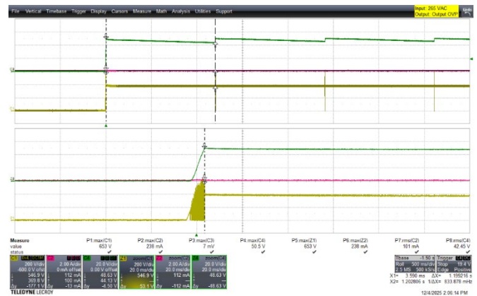
Figure 85 – 265 VAC, No Load – OVP during startup condition. CH1: TOP7075E_Vds, 200 V / div., 500 ms / div. CH2: Iout, 2 A / div., 500 ms / div. CH3: Vout, 20 V / div., 500 ms / div. Zoom: 20 ms/div. Maximum Output Voltage = 50.5 V.
