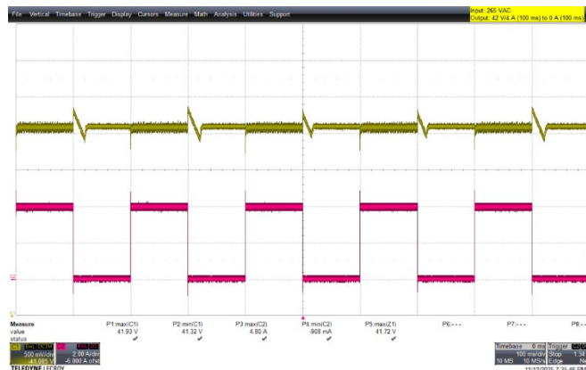
Figure 21 – 265 VAC, 50 Hz. I_o = 0 - 4 A (0-100%) load step.
