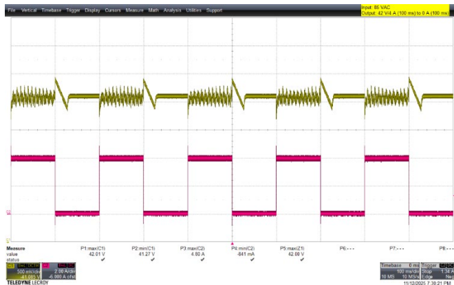
Figure 18 – 85 VAC, 60 Hz. I_o = 0 - 4 A (0-100%) load step.
