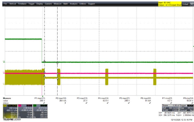
Figure 94 – 85 VAC, No Load – Output short circuit during normal condition.
