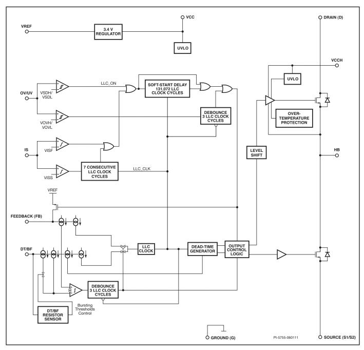
Figure 2. Block Diagram.
