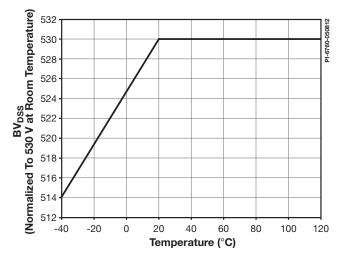
Figure 33. Normalized  $\mathrm{BV}_{\mathrm{DSS}}$  vs. Temperature.
