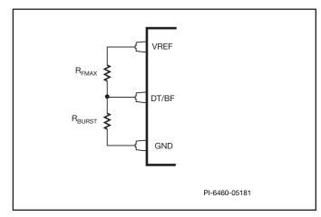
Figure 15. DT/BF Pin Divider.
