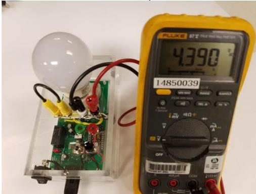
**Figure 14** – Leakage Voltage, Bulb is OFF.
