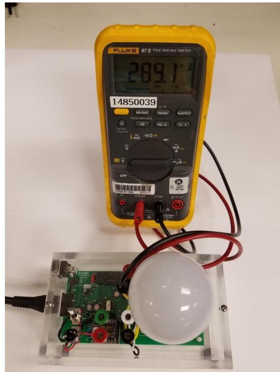
**Figure 12** – Input Current, With BLE Load, 230 VAC.
