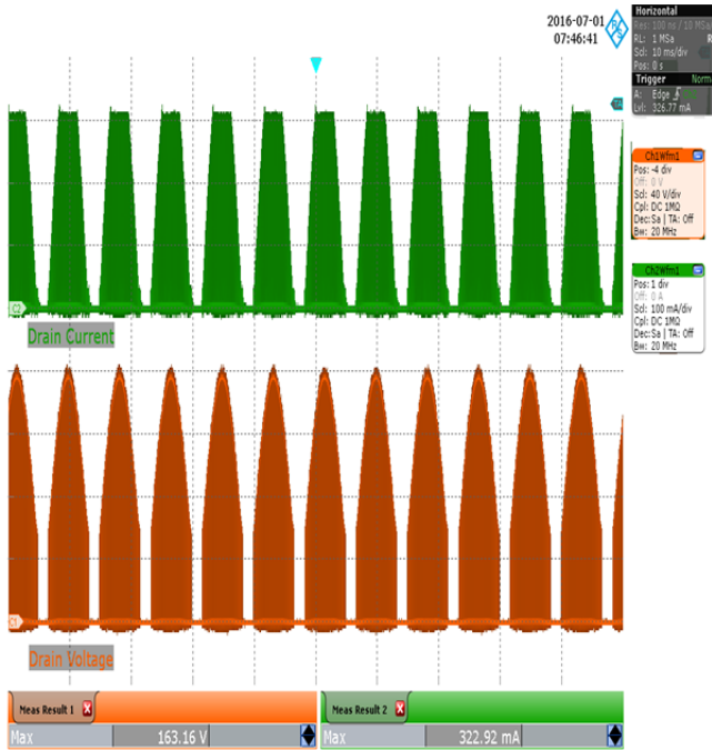
Figure 31 – 115 VAC, 52 V LED Load. Upper: I_{DRAIN} , 100 mA / div. Lower: V_{DRAIN} , 40 V / div., 10 ms / div. V_{DS(MAX)} : 163.16 V, I_{D(MAX)} : 322.92 mA
