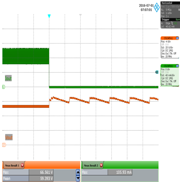
Figure 52 – 115 VAC, 52 V LED Load, Running then Open Load. Upper: I_{OUT} , 40 mA / div. Lower: V_{OUT} , 20 V / div., 1 s / div. V_{OUT(MAX)} : 66.561 V. V_{OUT(MEAN)} : 59.393 V.
