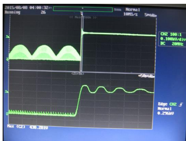
Figure 84 – +1000 kV Differential Surge, 90 °C Phase.
