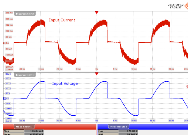
Figure 71 – 110° Conduction Angle. Upper: I_{IN} , 50 mA / div. Lower: V_{IN} , 50 V / div., 4 ms / div. Peak V_{IN} : 171.06 V. V_{RMS} : 98.766 V.
