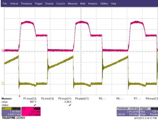
**Figure 25** – Main Stage Primary Voltage and Current, 115 VAC Input, 100% Load.
