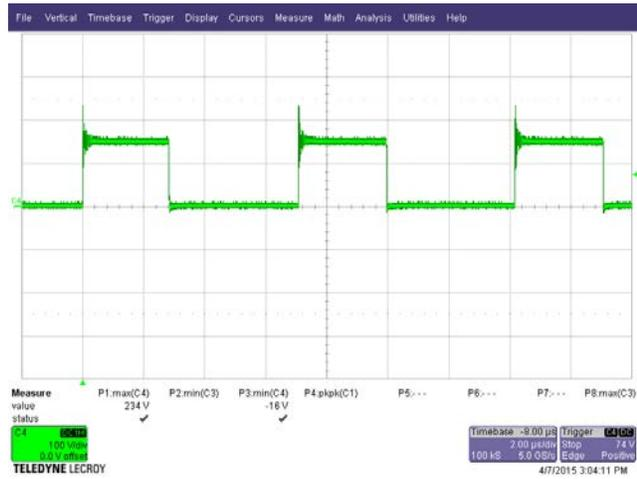
**Figure 28** – Output Catch Rectifier (D19) Reverse Voltage, 132 VAC, 100% Load. 100 V, 2 µs / div.
