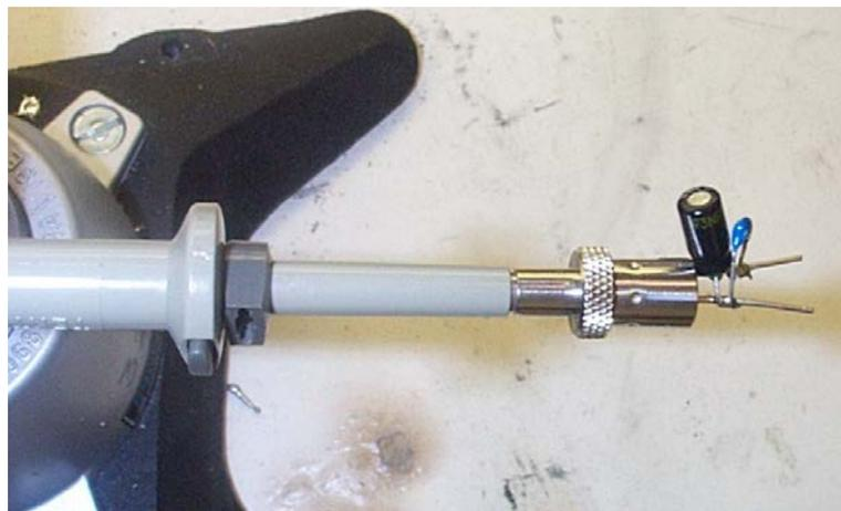
**Figure 43** – Oscilloscope Probe with Probe Master 4987BA BNC Adapter (Modified with Wires for Probe Ground for Ripple measurement and Two Parallel Decoupling Capacitors Added).
