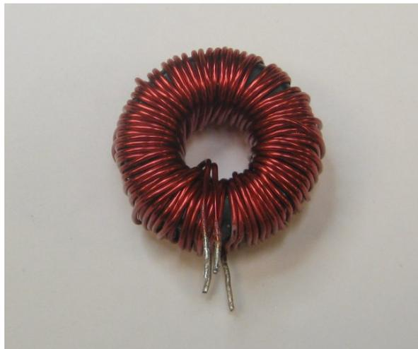
Figure 10 – Finished Output Choke.
