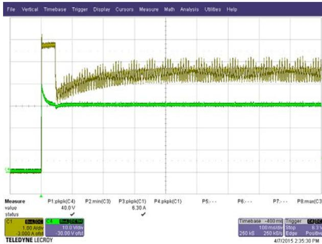
**Figure 32** – Main Output Start-up, Constant Current Mode, 115 VAC, Chroma CV Load, 30 V Setting.
