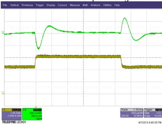
**Figure 40** – Main Output Transient Response, CV Mode, 50%-75%-50% Load Step, 115 VAC Input.
