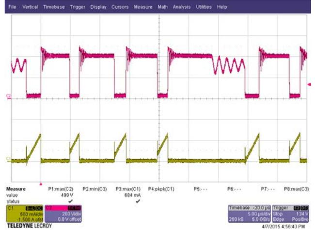
**Figure 26** – Standby Primary Voltage and Current, 115 VAC Input, 100% Load.
