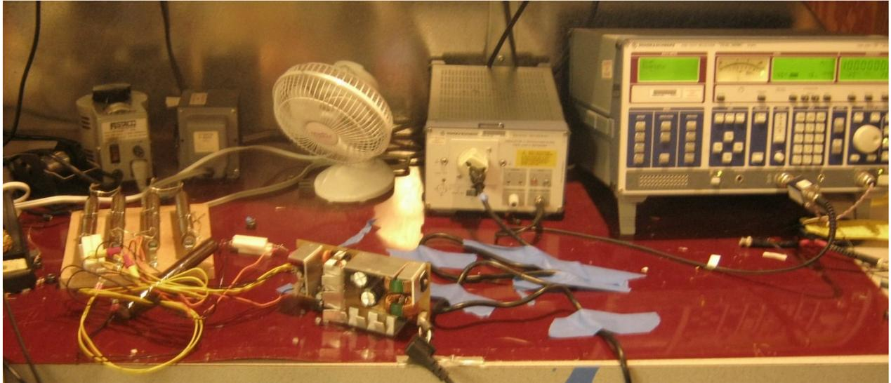
**Figure 53** – EMI Set-up with Floating Resistive Load.
