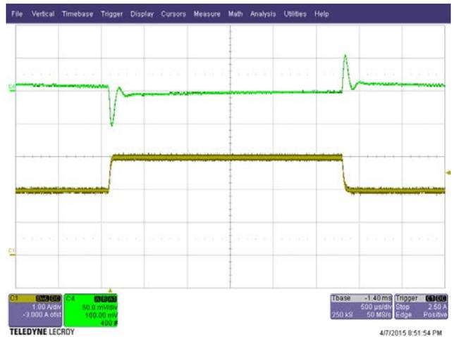
**Figure 41** – Standby Output Transient Response, CV Mode, 50%-75%-50% Load Step, 115 VAC Input.
