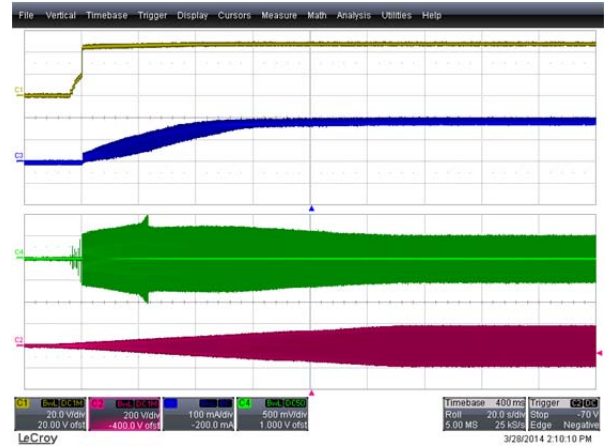
Figure 51 – 48 V Output, Brown-in Condition (1 V / s Ramp Rate). CH1: V_{OUT} , 20 V / div. CH2: V_{IN} , 200 V / div. CH3: I_{OUT} , 100 mA / div. CH4: I_{IN} , 500 mA, 20 s / div.
