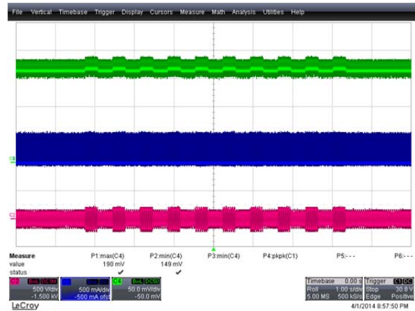
Figure 55 – 90 VAC to 132 VAC Line Transient. CH2: V_{IN} , 500 V / div. CH3: I_{DRAIN} , 500 mA / div. CH4: I_{OUT} , 50 mA / div., 1 s / div.
