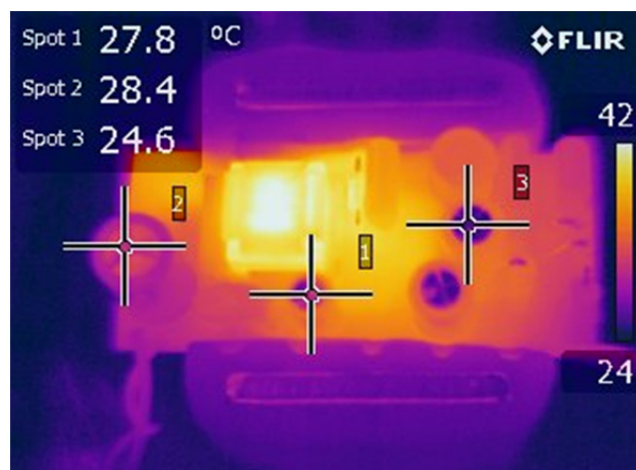
Figure 17 – Top side component guide for thermal scan.
