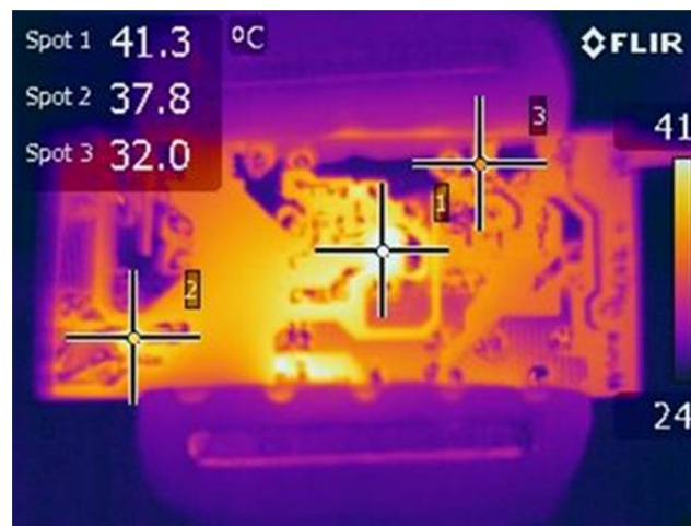
Figure 21 – SP1 – LYT2003D (U1). SP2 – Output Diode (D11). SP3 – Bridge Diode (D2).
