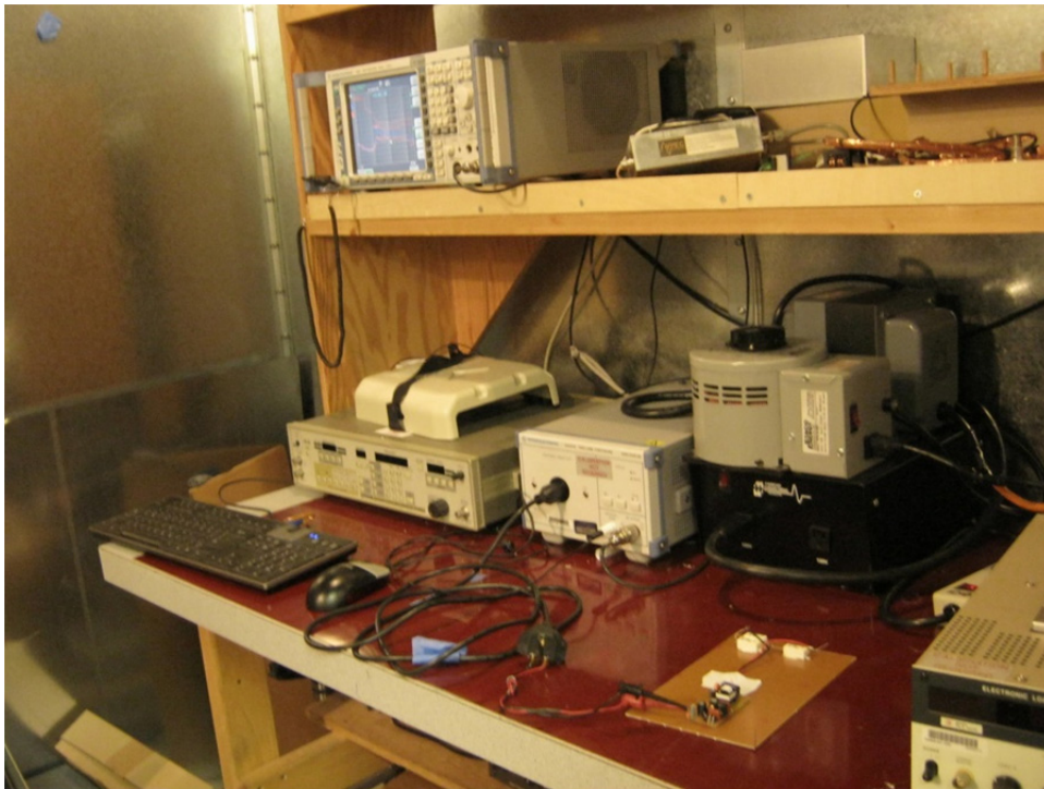
Figure 92 – Conducted EMI Set-up.
