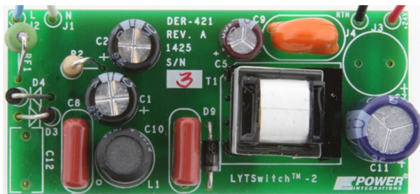
Figure 22 – Top side component guide for thermal scan.
