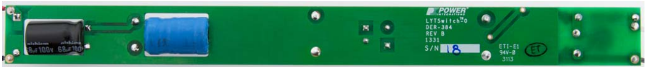
Figure 5 – Populated Circuit Board, D Package, Bottom.
