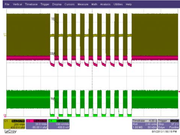
Figure 50 – Line Sag Test at 230 - 0 V at 0.5 s Interval. Ch1:V IN , 200 V / div. Ch2:V OUT , 20 V / div. Ch4:I OUT , 100 mA / div. Time Scale:2 s / div.
