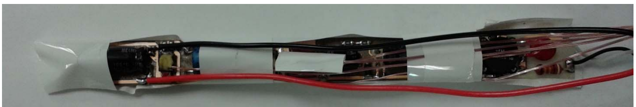
Figure 18 – Thermal Unit with Thermocouple Set-up.
