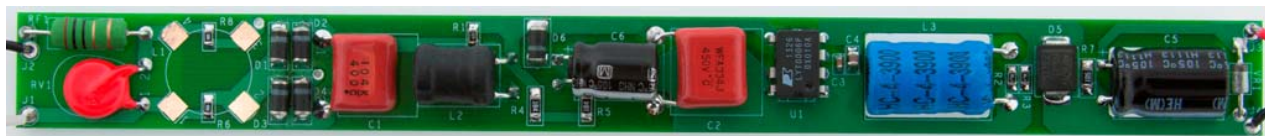
Figure 2 – Populated Circuit Board, P Package, Top.
