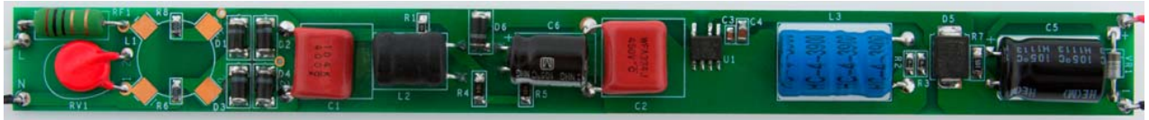
Figure 4 – Populated Circuit Board, D Package, Top.
