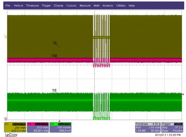
Figure 52 – Line Sag Test at 230 - 0 V at 0.1 s Interval. Ch1:V IN , 200 V / div. Ch2:V OUT , 20 V / div. Ch4:I OUT , 100 mA / div. Time Scale:2 s / div.
