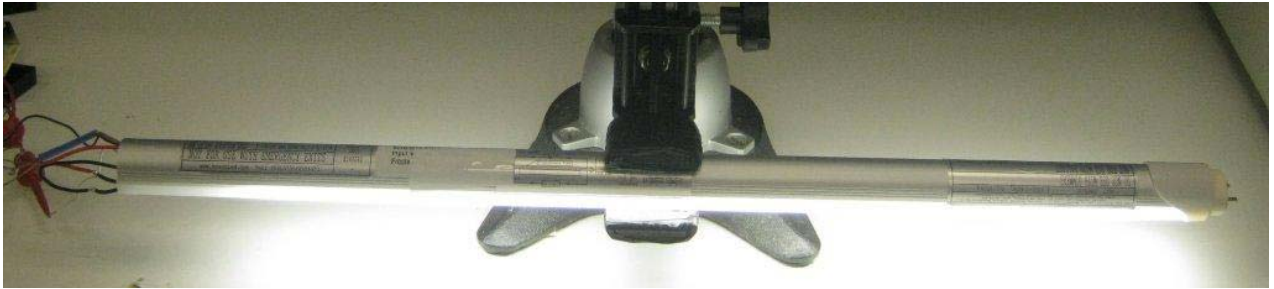
Figure 16 – LED Driver Inserted in a T8, 2 ft. Tube for Thermal Evaluation.
