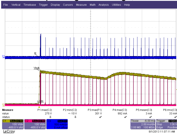
Figure 33 – LYT0006D Output Short.190 VAC. Ch1:V BULK , 100 V / div. Ch2:V S-G , 100 V / div. Ch3:I DRAIN , 0.5 A / div. Time Scale:2 ms / div.
