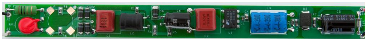
Figure 2 – Populated Circuit Board, P Package, Top.
