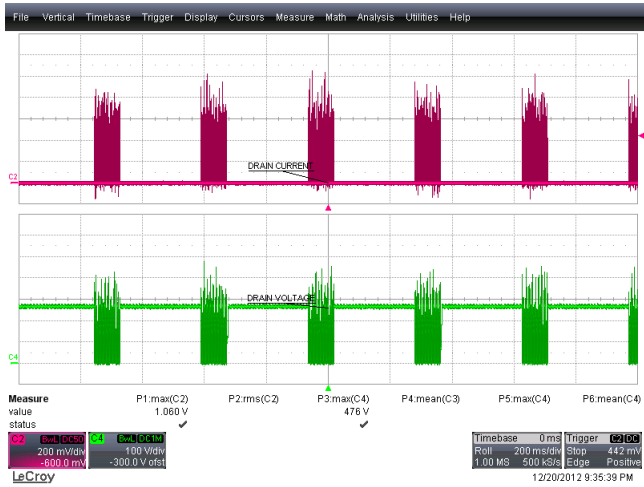
Figure 41 – 190 VAC, 50 Hz Output Short Condition. Upper: I_{DRAIN} , 200 mA / div. Lower: V_{DRAIN} , 100 V, 200 ns / div.
