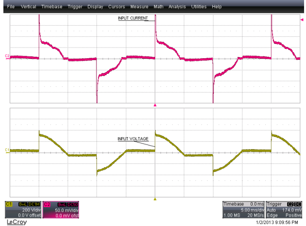
Figure 58 – 90° Conduction Angle. Upper: I_{IN} , 50 mA / div. Lower: V_{IN} , 200 V, 5 ms / div.
