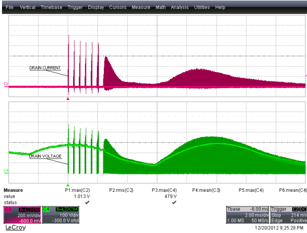
Figure 37 – 190 VAC, 50 Hz Start-up. Upper: I_{DRAIN} , 200 mA / div. Lower: V_{DRAIN} , 100 V, 2 ms / div.
