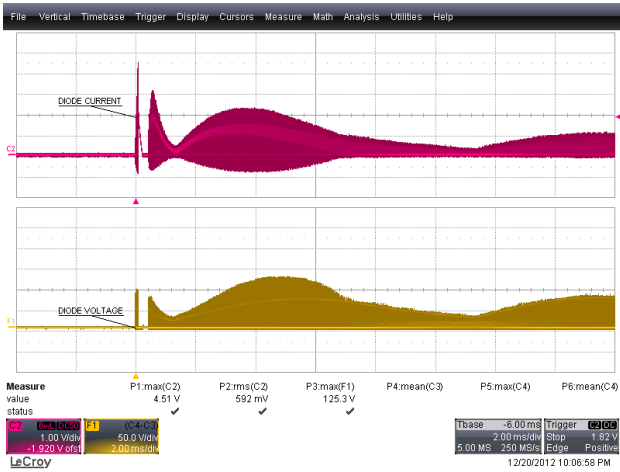
Figure 49 – 190 VAC, 50 Hz. Upper: I_{D7} , 1 A / div. Lower: V_{D7} , 50 V, 2 ms / div.
