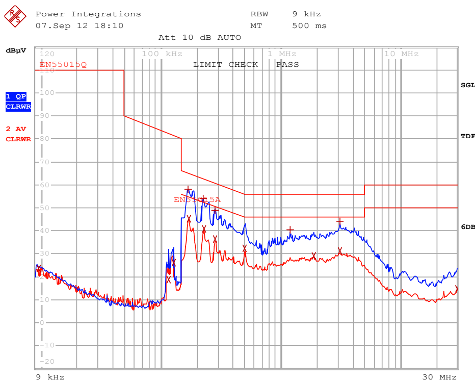
Figure 46 – Conducted EMI 9 V / 330 mA Load, 115 VAC, 60 Hz, and EN55015 Limits.
