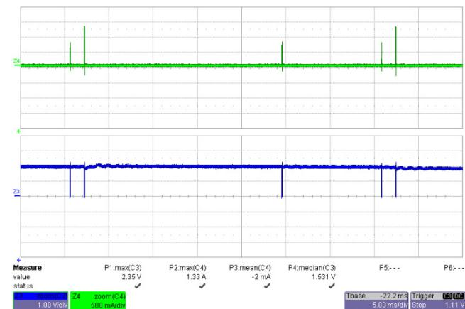
**Figure 45 – 135 VAC, 60 Hz Output Short Condition.**
