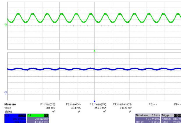
**Figure 19 – 100 VAC, 60 Hz Full Load.**
