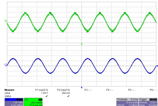
Figure 15 – 100 VAC, 60 Hz Full Load.
