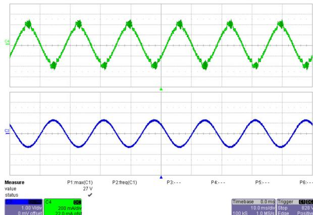
Figure 14 – 90 VAC, 60 Hz Full Load.
