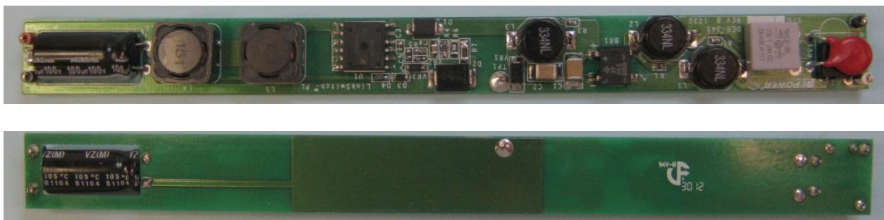
**Figure 1 – Populated Circuit Board (180 mm x 16.4 mm x 8 mm).**
