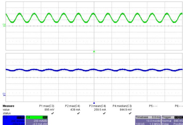
**Figure 20 – 115 VAC, 60 Hz Full Load.**
