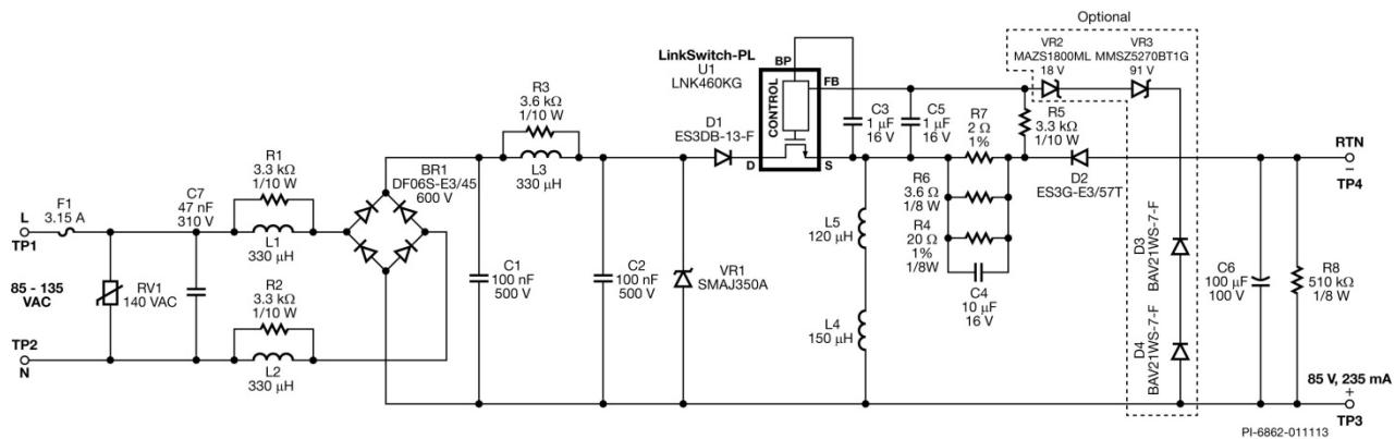
Figure 2 – Schematic.
