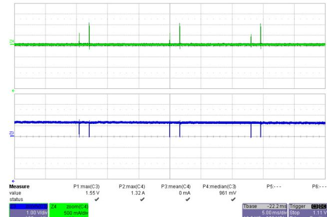
**Figure 43 – 90 VAC, 60 Hz Output Short Condition.**
