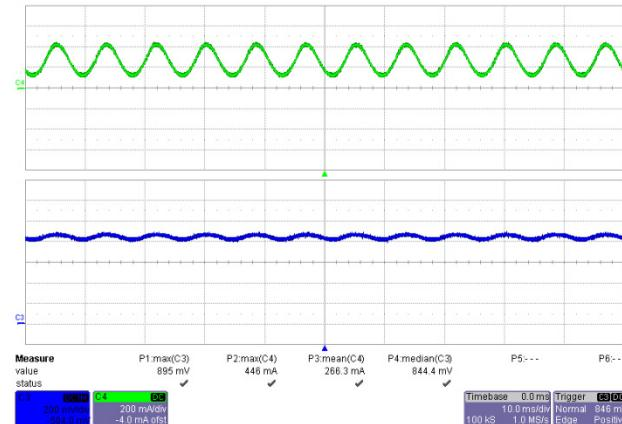
**Figure 21 – 135 VAC, 60 Hz Full Load.**
