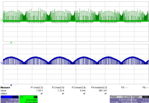
**Figure 42 – 90 VAC, 60 Hz Output Short Condition.**
