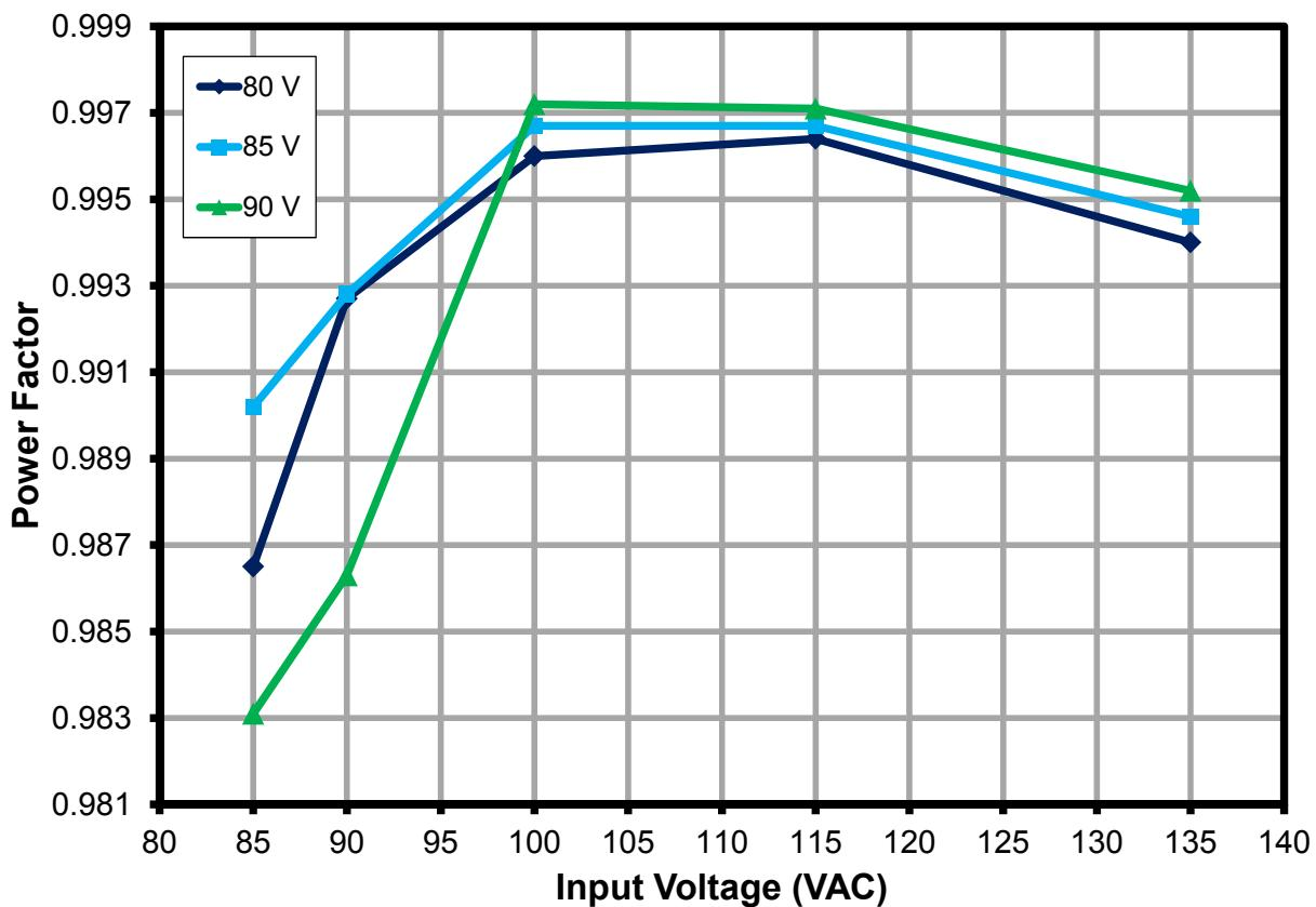
**Figure 7 – Power Factor vs. Line and Load.**
