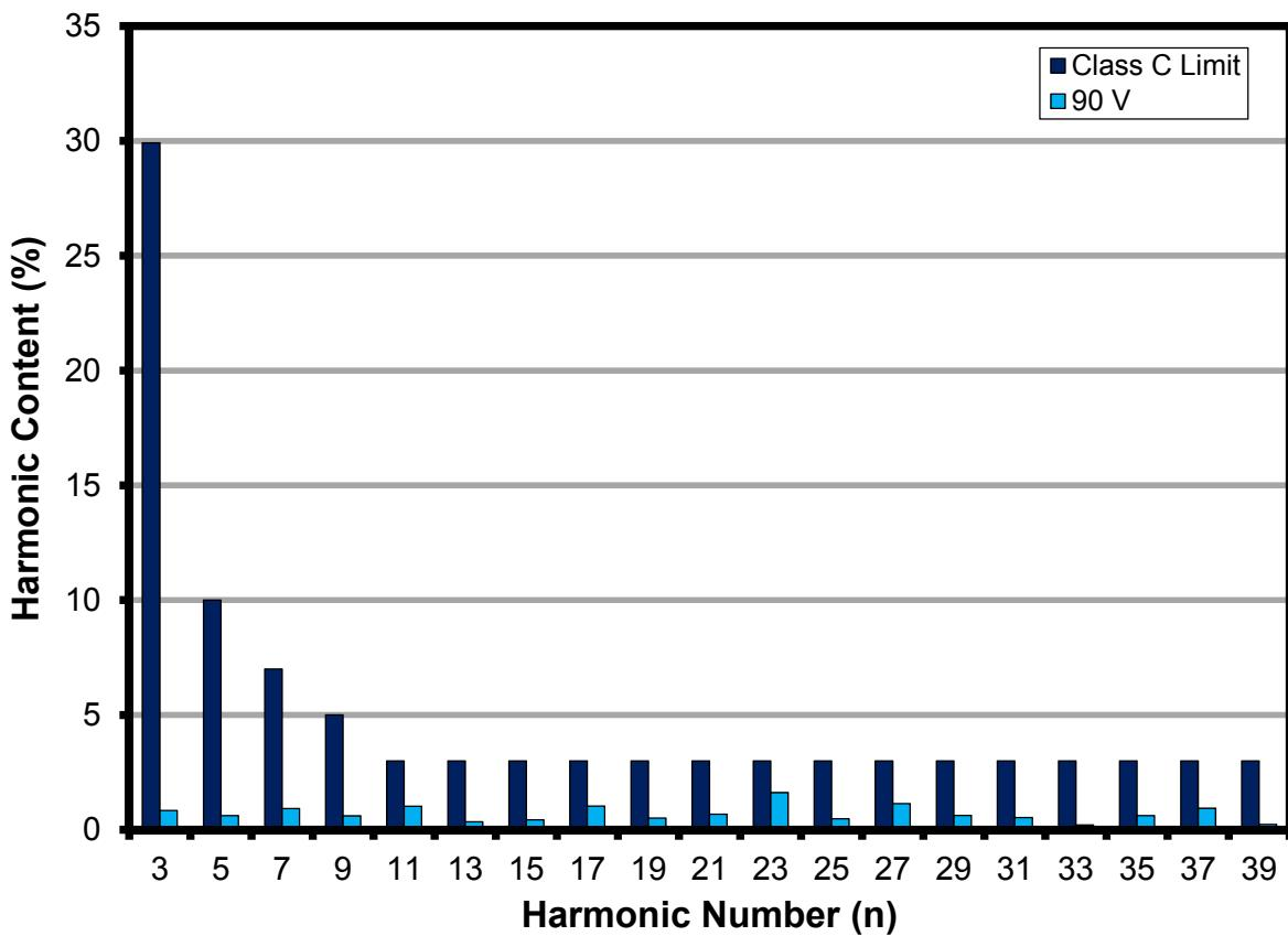
**Figure 11 – 90 V Output. Input Current Harmonics (IEC 61000-3-2 Class C) at 115 VAC, 60 Hz.**
