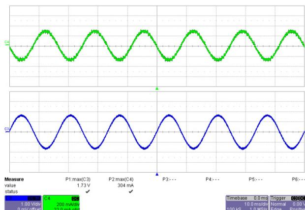
Figure 16 – 115 VAC, 60 Hz Full Load.
