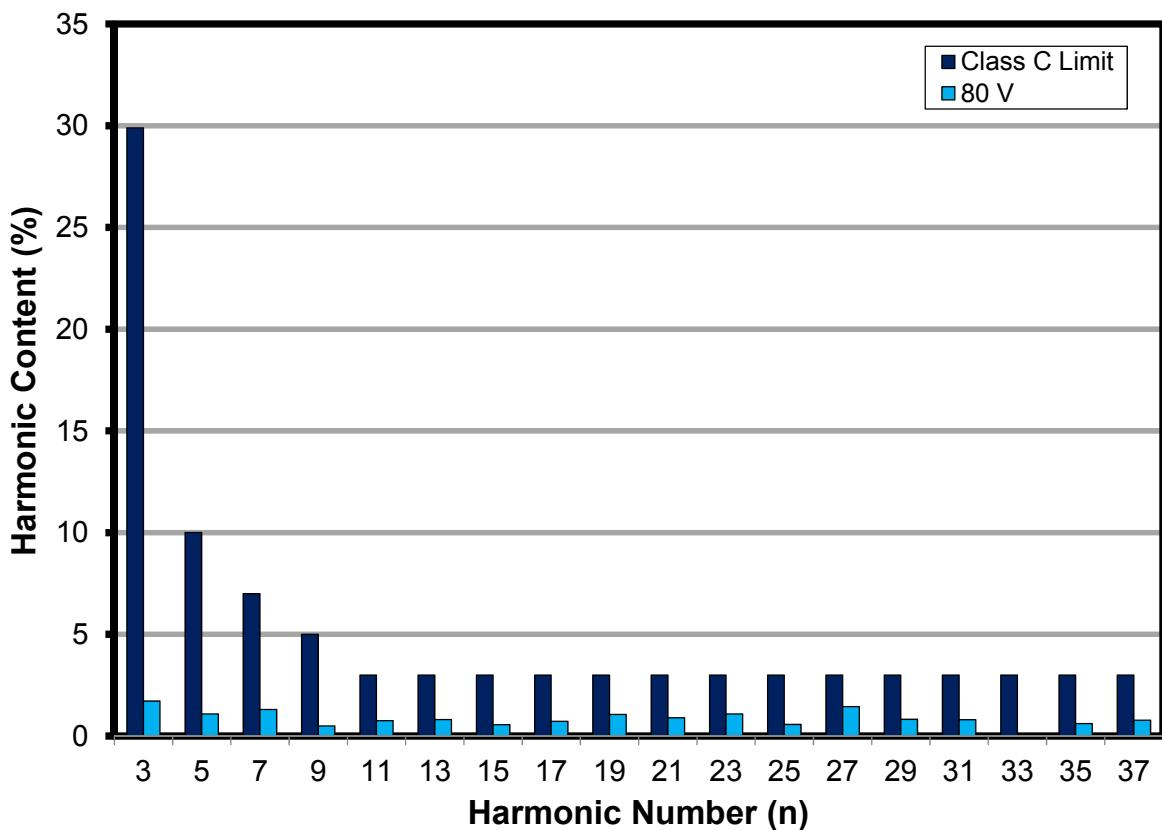
**Figure 9 – 80 V Output. Input Current Harmonics (IEC 61000-3-2 Class C) at 115 VAC, 60 Hz.**
