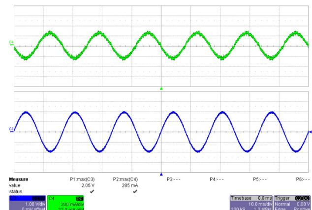
Figure 17 – 135 VAC, 60 Hz Full Load.
