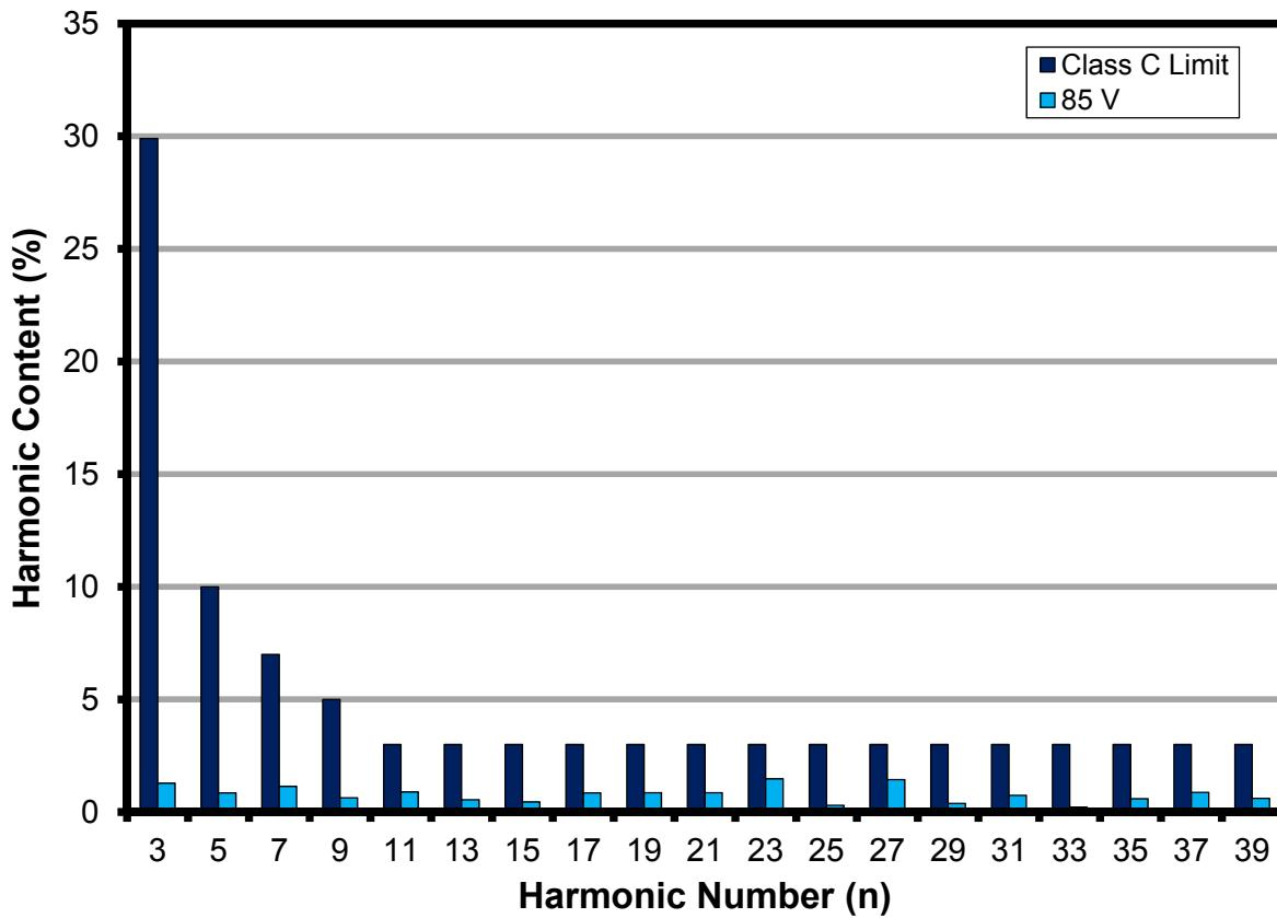
Figure 10 – 85 V Output. Input Current Harmonics (IEC 61000-3-2 Class C) at 115 VAC, 60 Hz.
