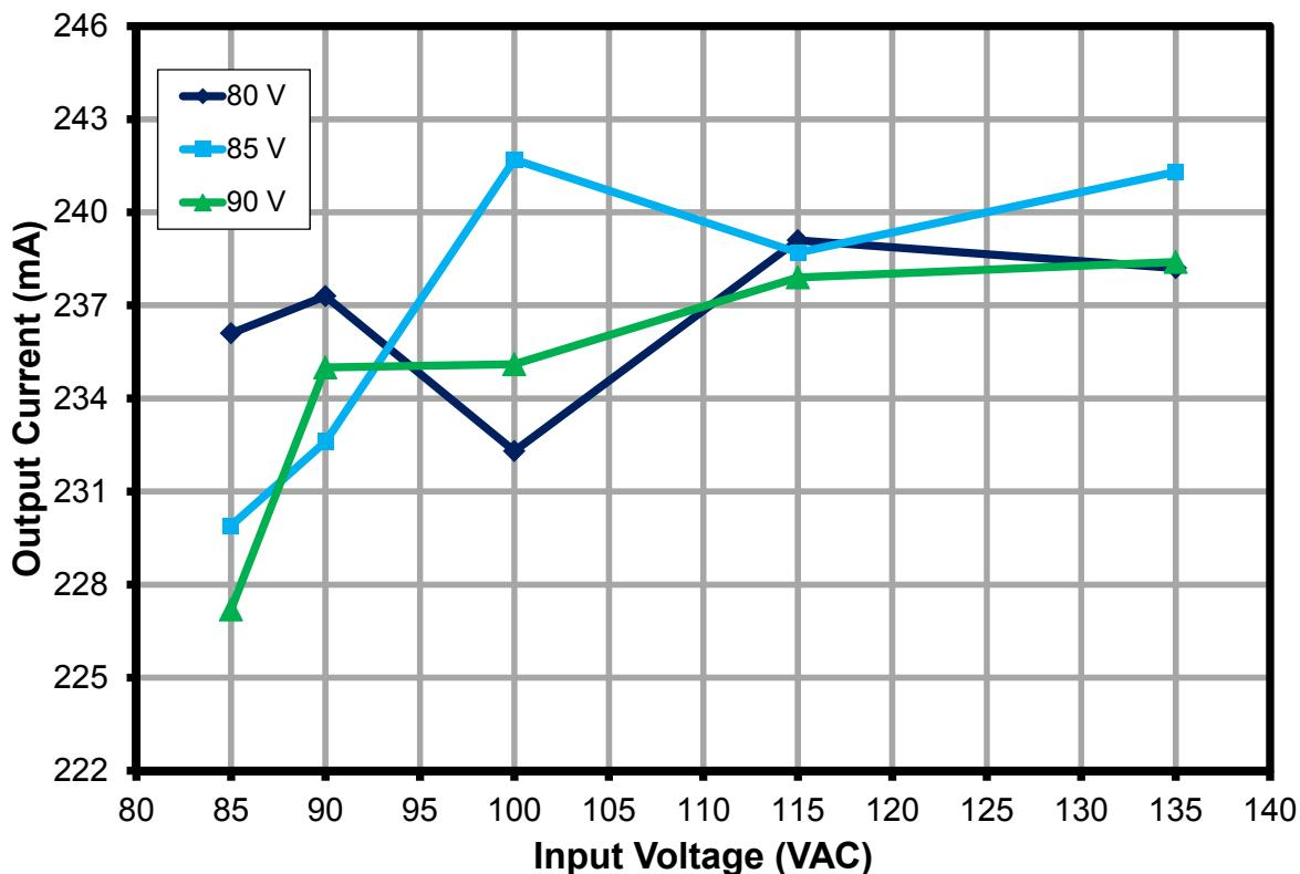
Figure 6 – Regulation vs. Line and Load.
