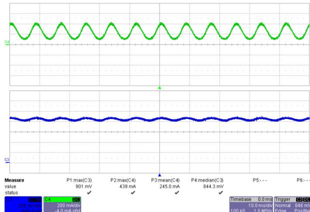
**Figure 18 – 90 VAC, 60 Hz Full Load.**
