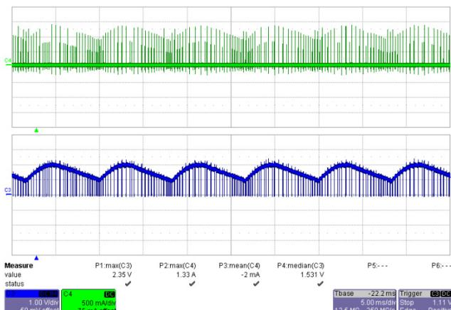
**Figure 44 – 135 VAC, 60 Hz Output Short Condition.**
