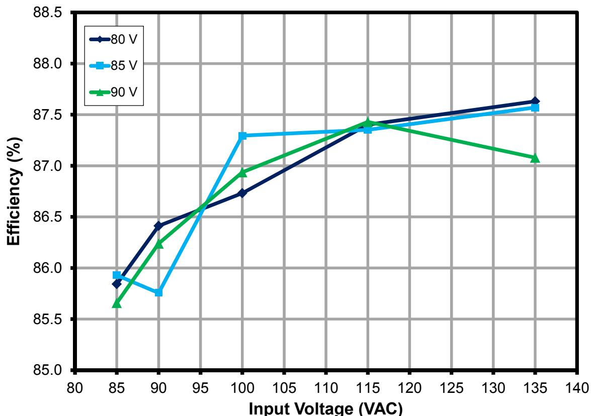
**Figure 5 – Efficiency vs. Line and Load.**
