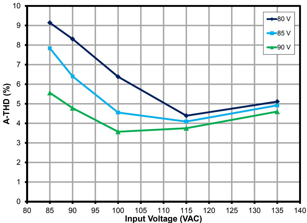
Figure 8 – A-THD vs. Line and Load.
