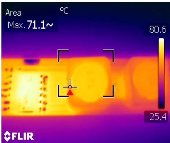
Figure 12 – Output Inductor: 71 °C.
