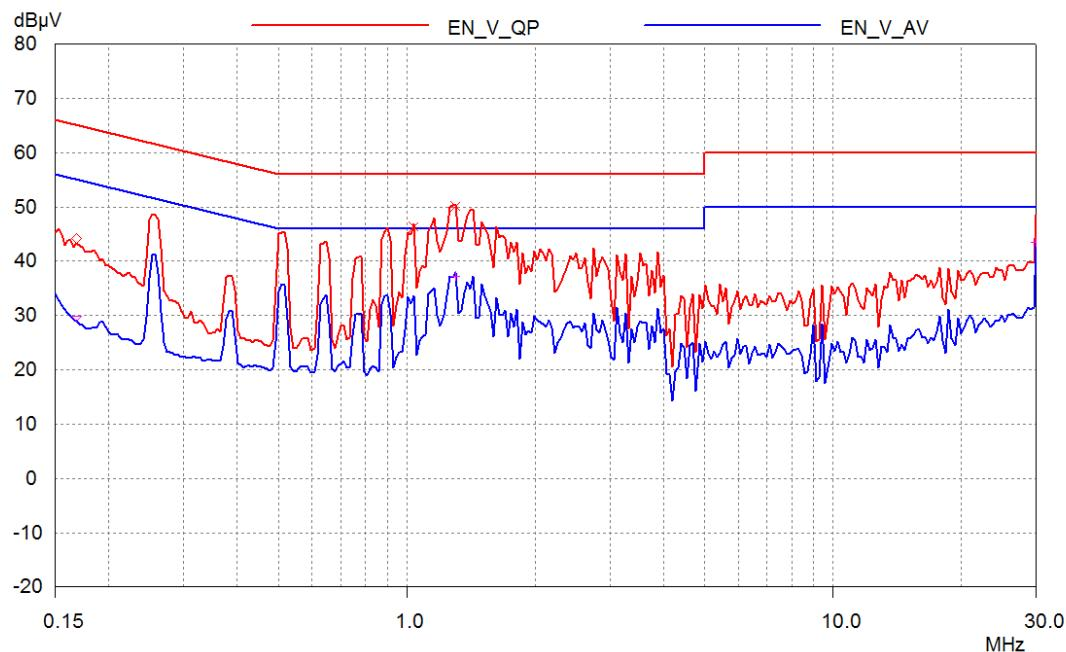
**Figure 46 –** Conducted EMI 85 V / 235 mA Load, 115 VAC, 60 Hz, and EN55015 Limits.
