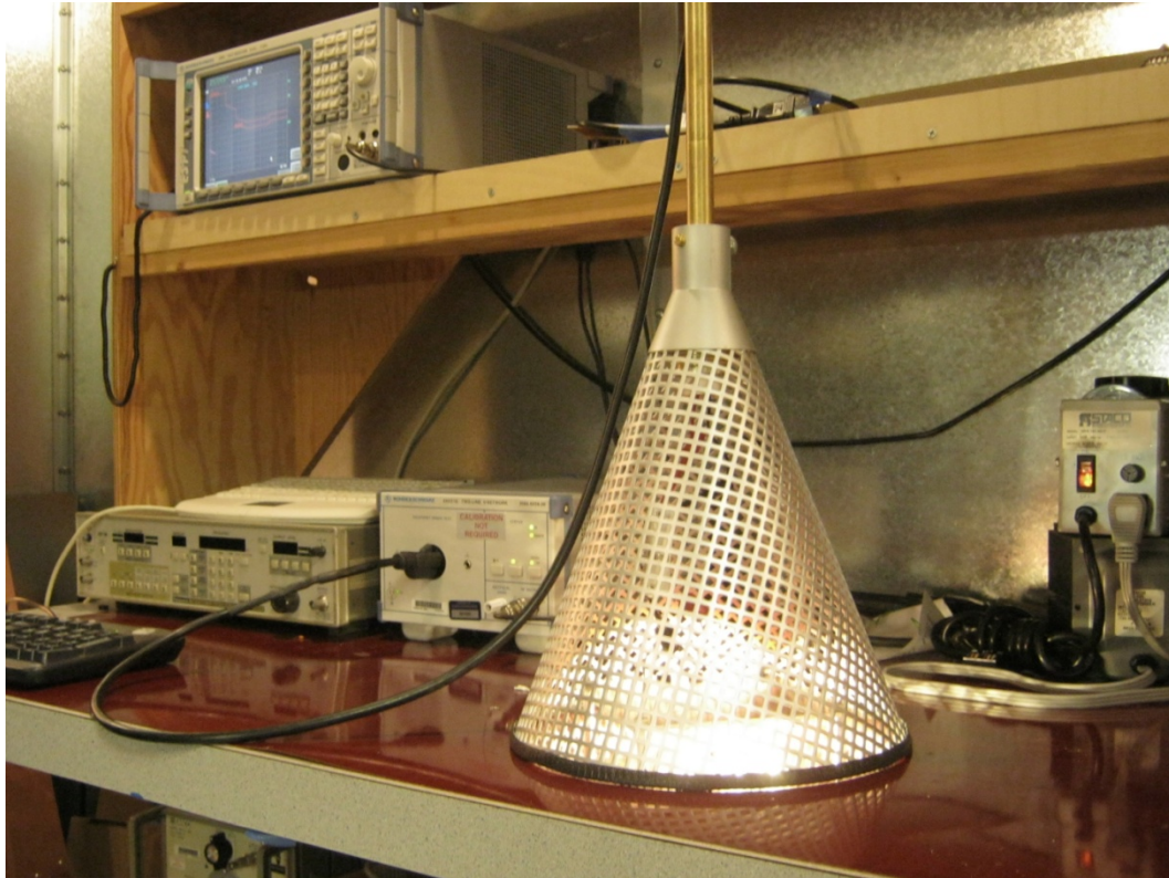
Figure 65 – EMI Set-up: LED Driver and Load were Placed Inside the Cone.
