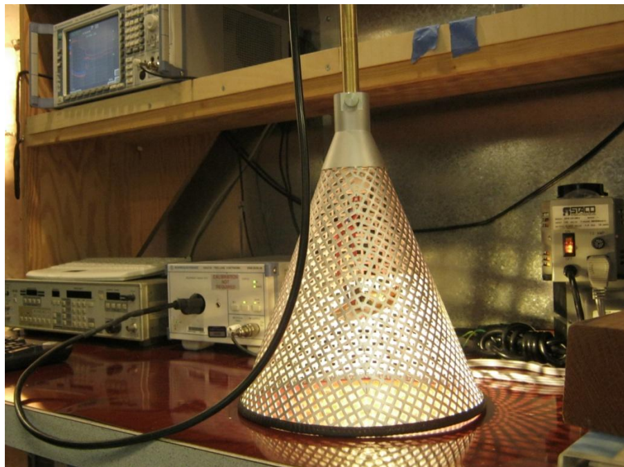
Figure 60 – EMI Test Set-up with the Unit and LED Load Placed Inside the Cone.
