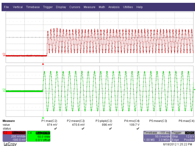
Figure 37 – 110 VAC, 60 Hz. Upper: I_{OUT} , 200 mA / div. Lower: V_{IN} , 50 V, 50 ms / div.
