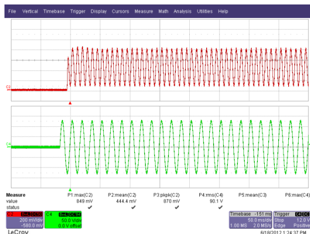
Figure 36 – 90 VAC, 60 Hz. Upper: I_{OUT} , 200 mA / div. Lower: V_{IN} , 50 V, 50 ms / div.
