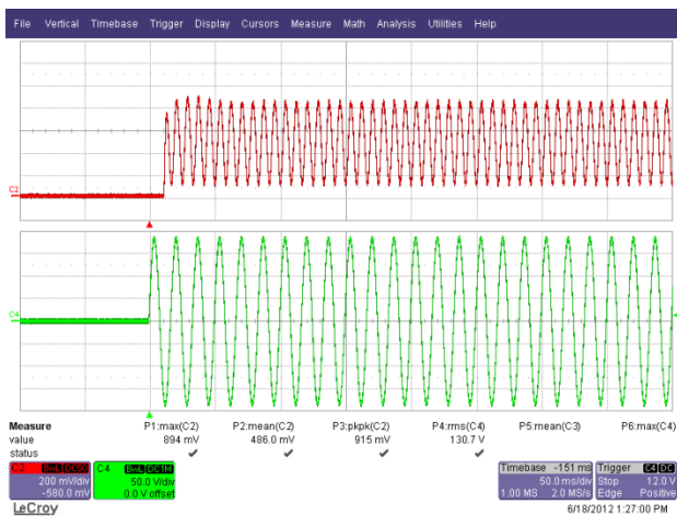
Figure 39 – 132 VAC, 60 Hz. Upper: I_{OUT} , 200 mA / div. Lower: V_{IN} , 50 V, 50 ms / div.
