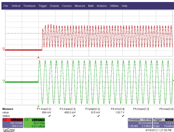
Figure 39 – 132 VAC, 60 Hz. Upper: I_{OUT} , 200 mA / div. Lower: V_{IN} , 50 V, 50 ms / div.
