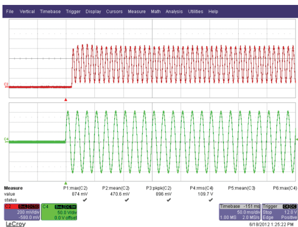
Figure 37 – 110 VAC, 60 Hz. Upper: I_{OUT} , 200 mA / div. Lower: V_{IN} , 50 V, 50 ms / div.
