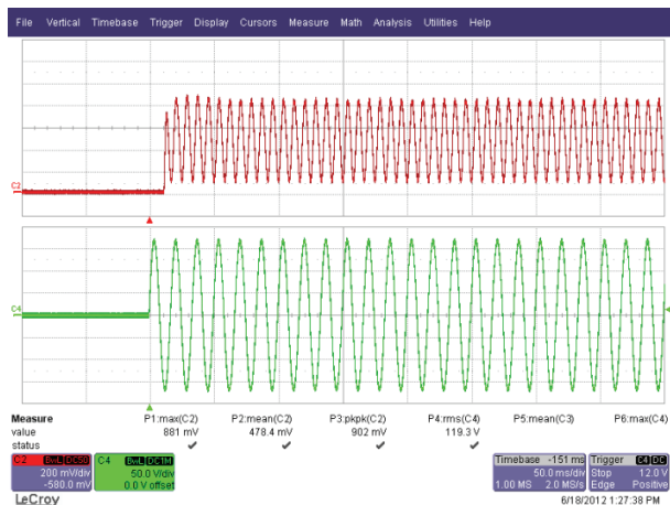
Figure 38 – 120 VAC, 60 Hz. Upper: I_{OUT} , 200 mA / div. Lower: V_{IN} , 50 V, 50 ms / div.
