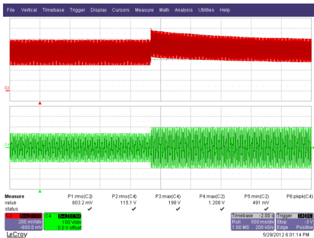
Figure 46 – 90 VAC – 132 VAC, 60 Hz. Upper: I_{OUT} , 200 mA / div. Lower: V_{IN} , 100 V / div., 500 ms / div. I_{OUT} Peak: 1.21 A.
