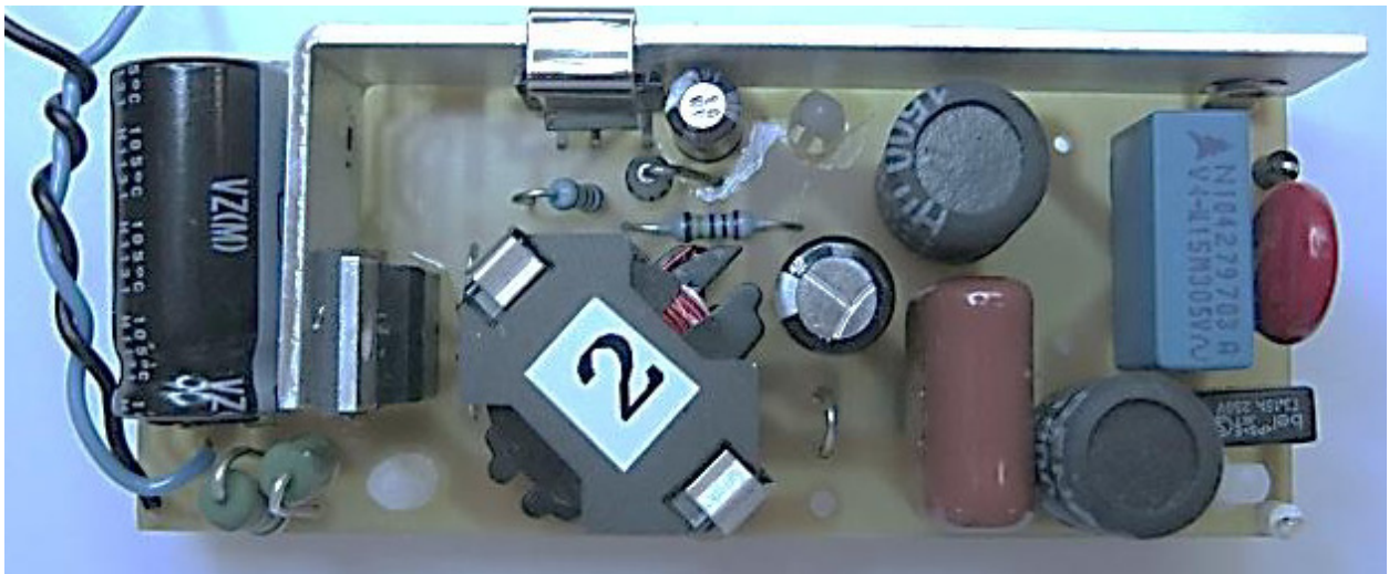
Figure 2 – Populated Circuit Board (Top View), 86 mm x 36 mm.
