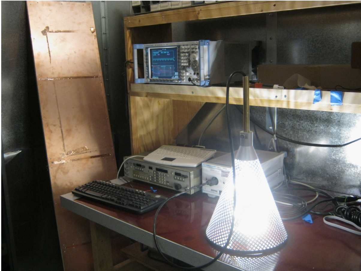
Figure 56 – EMI Set-up: LED Driver and Load were Placed Inside the Cone.
