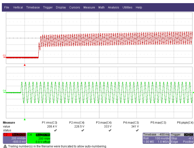
Figure 40 – 230 VAC Full Load. Upper: I_{OUT} , 200 mA / div. Lower: V_{IN} , 200 V / div., 100 ms / div.
