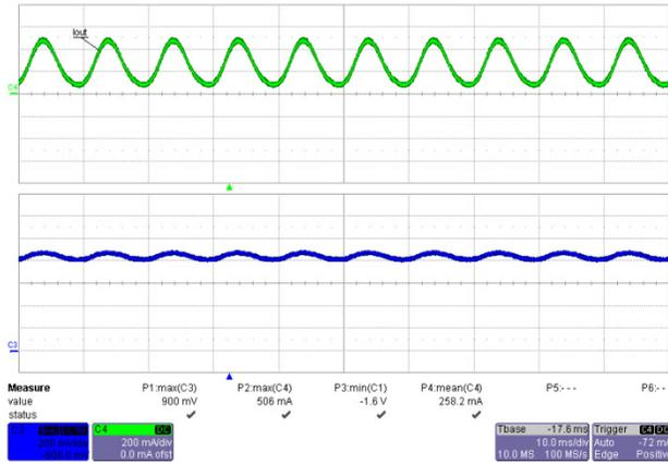
**Figure 17 – 195 VAC, 50 Hz Full Load.**
