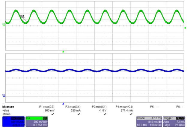
**Figure 18 – 210 VAC, 50 Hz Full Load.**
