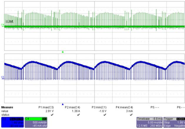
**Figure 39** – 195 VAC, 50 Hz Output Short Condition.
