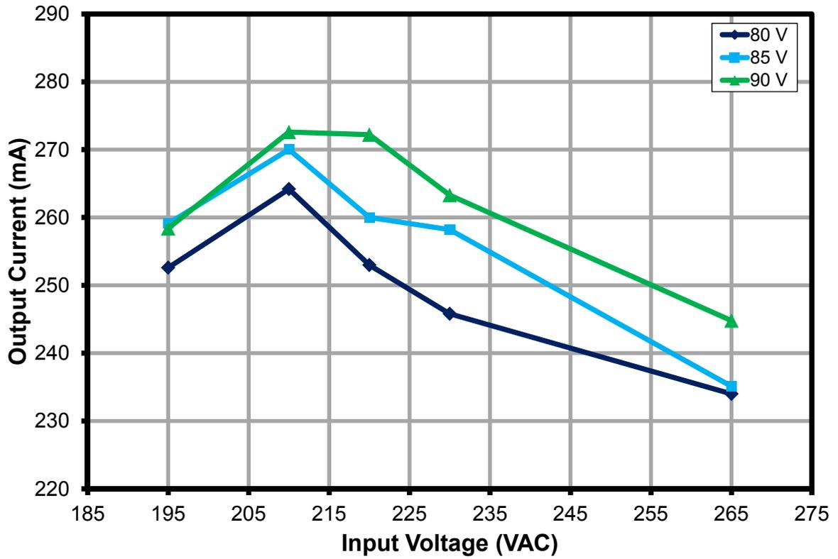
Figure 5 – Regulation vs. Line and Load.
