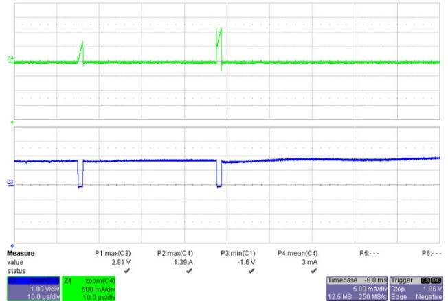
**Figure 40** – 195 VAC, 50 Hz Output Short Condition.
