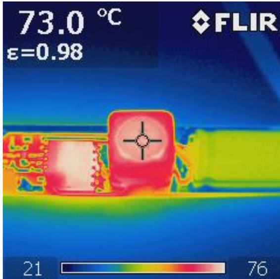
Figure 11– Output Inductor: 73 °C.
