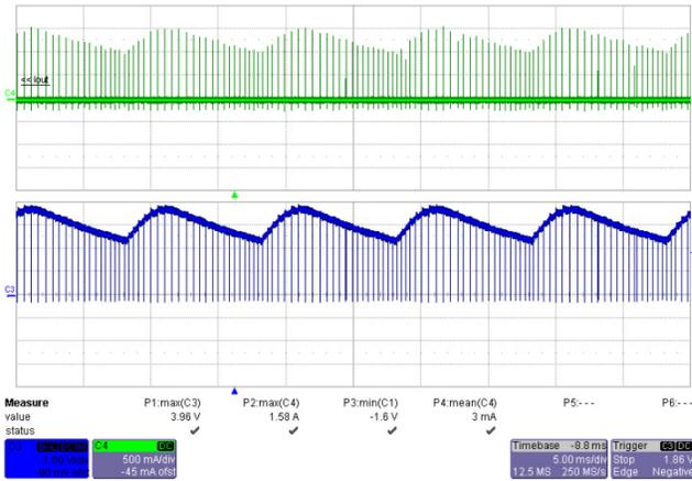
**Figure 41** – 265 VAC, 50 Hz Output Short Condition.
