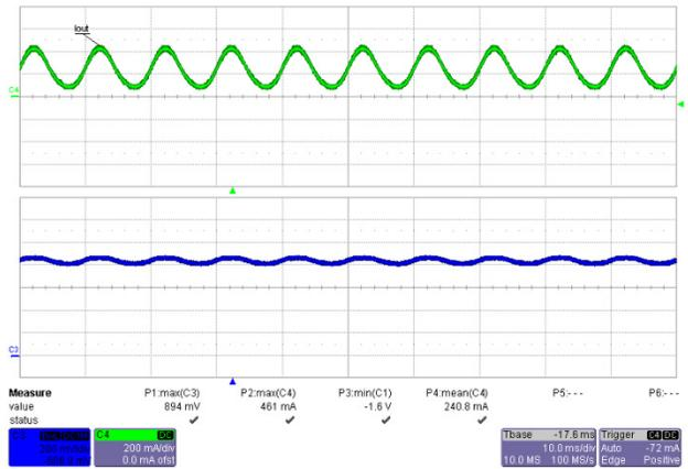
**Figure 20 – 265 VAC, 50 Hz Full Load.**
