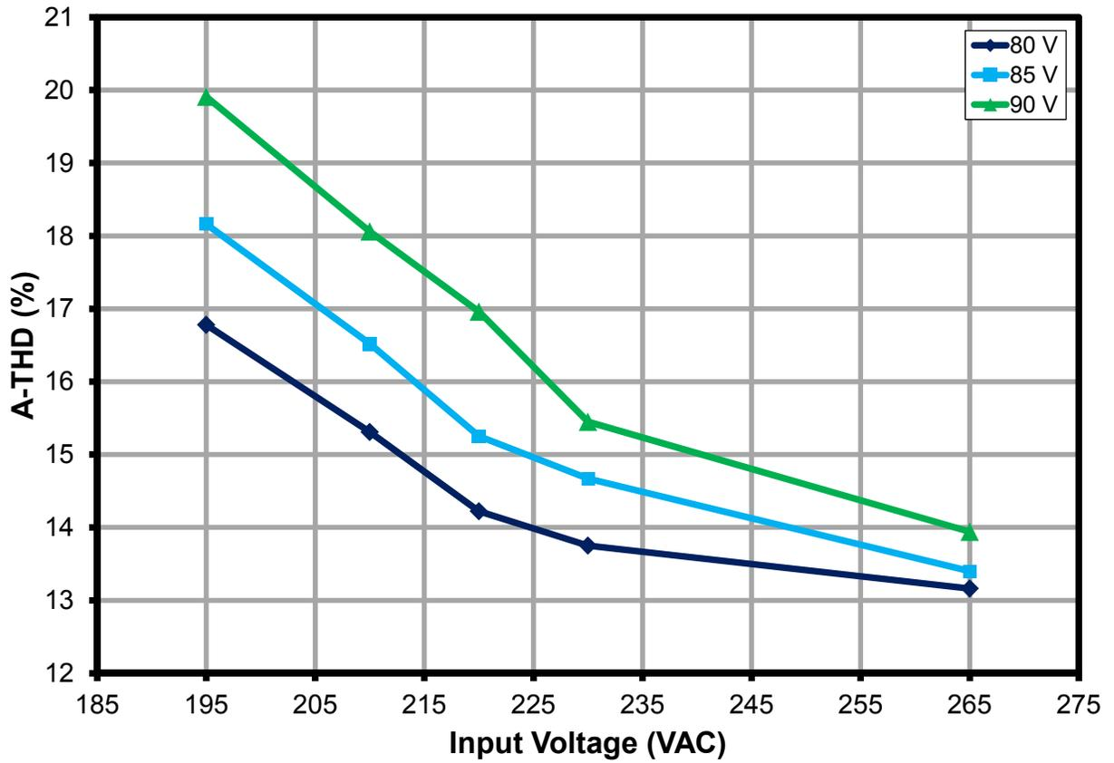
Figure 7 – A-THD vs. Line and Load.
