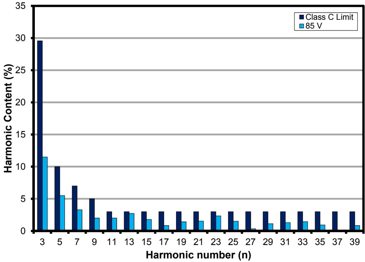
Figure 9 – 85 V Output. Input Current Harmonics at 230 VAC, 50 Hz.
