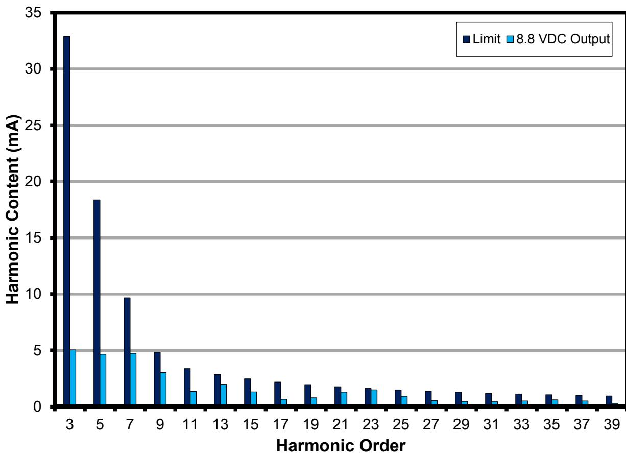
**Figure 13 – Meets EN61000-3-2 Harmonics Contents Standards for <25 W Rating for 230 V LED Output.**
