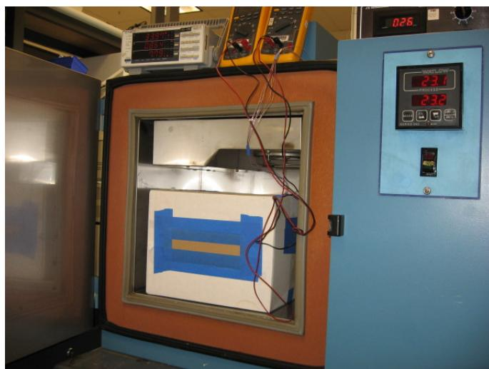
**Figure 16 – Thermal Chamber Set-up Showing Box Used to Prevent Airflow Over UUT.**
