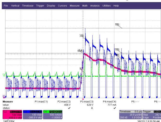
**Figure 55 – 230 VAC / 60 Hz, 9 V Load,**
