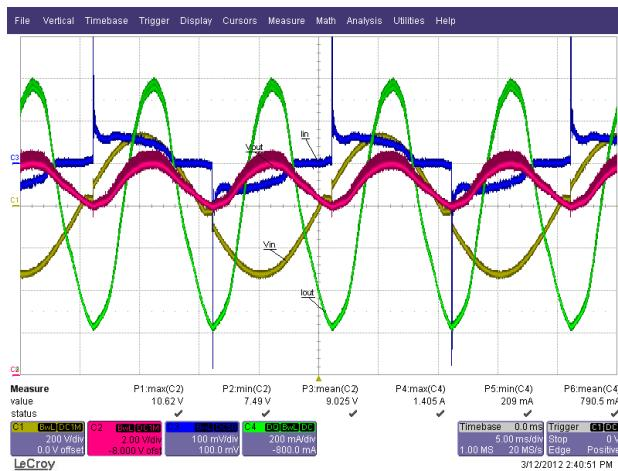
**Figure 47 – 230 VAC / 50 Hz, Sen Bo Lang Chinese Dimmer at Full TRIAC Conduction.**
