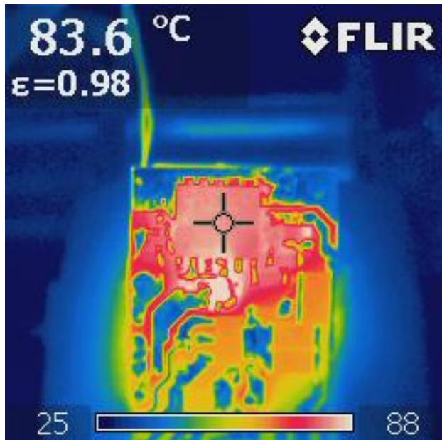
Figure 17 – LNK458KG U1 Case Temperature.
