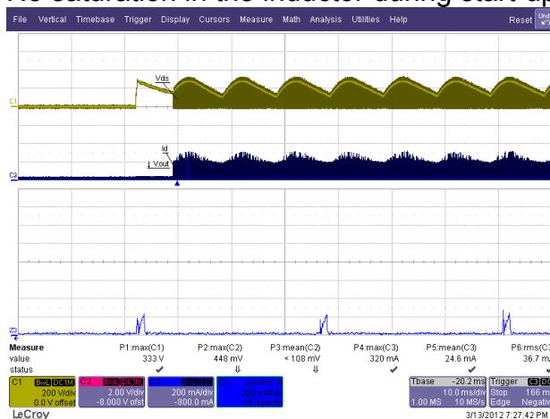
Figure 39 – 190 VAC / 50 Hz, Output Shorted.
