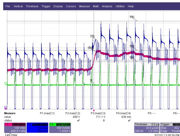
**Figure 56 – 230 VAC / 60 Hz, 9 V Load,**
