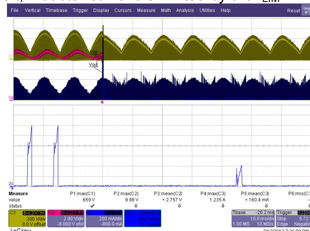
Figure 36 – 265 VAC / 50 Hz, Normal Operation then Output Short.
