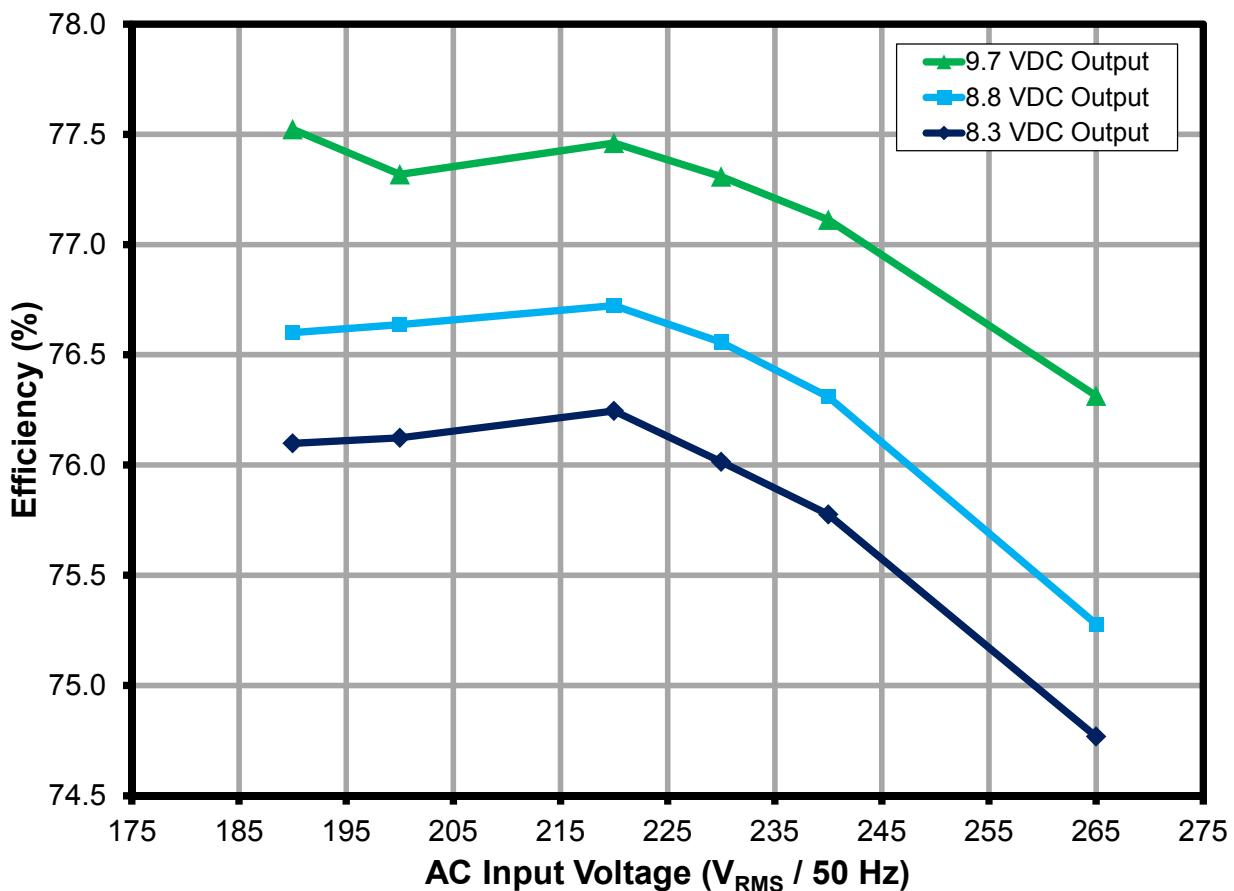
**Figure 9 – Efficiency with Respect to AC Input Voltage at 30 mA.**
