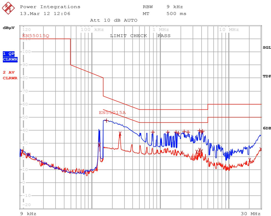
**Figure 60 –** Conducted EMI, 9 V Output / 800 mA Steady-State Load, 230 VAC, 60 Hz, and EN55015 Limits.
