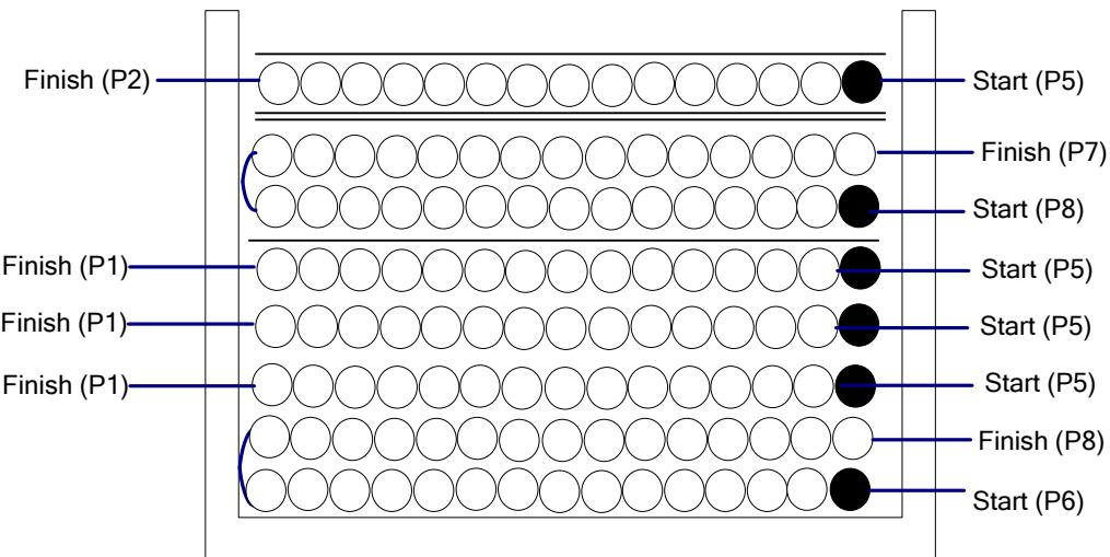
**Figure 8 – Transformer Build Diagram.**
