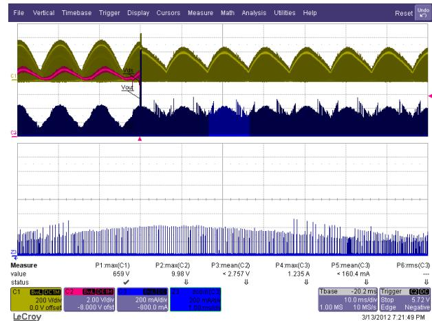
Figure 38 – 265 VAC / 50 Hz, Normal Operation then Output Short.
