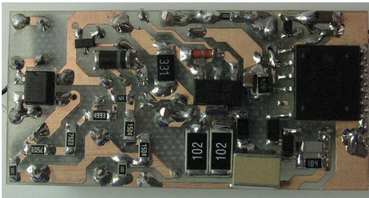
Figure 6 – Populated Circuit Board (bottom side).
