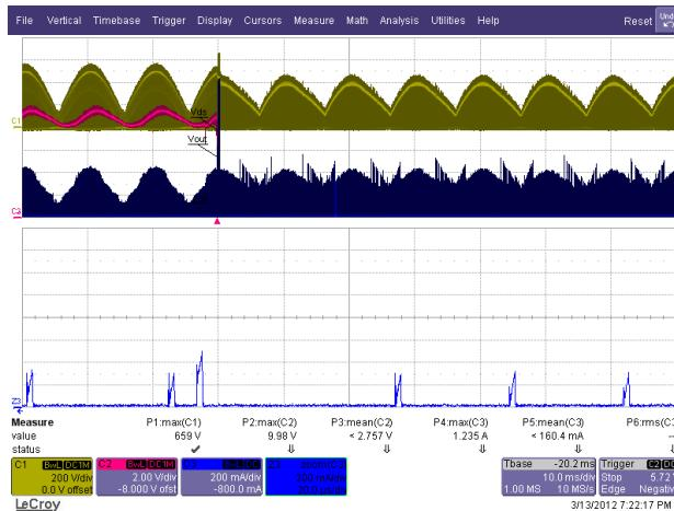
Figure 37 – 265 VAC / 50 Hz, Normal Operation then Output Short.
