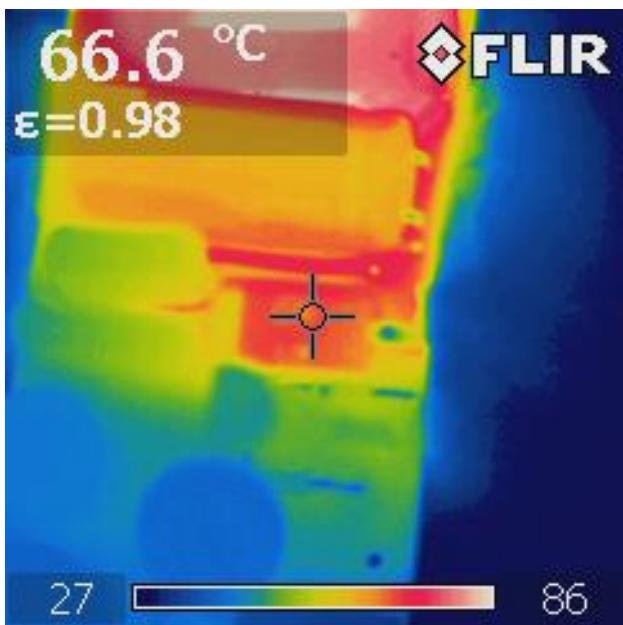
Figure 21 – D4 Output Diode.
