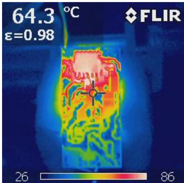
Figure 19 – Damper FET Q3 Case Temperature.
