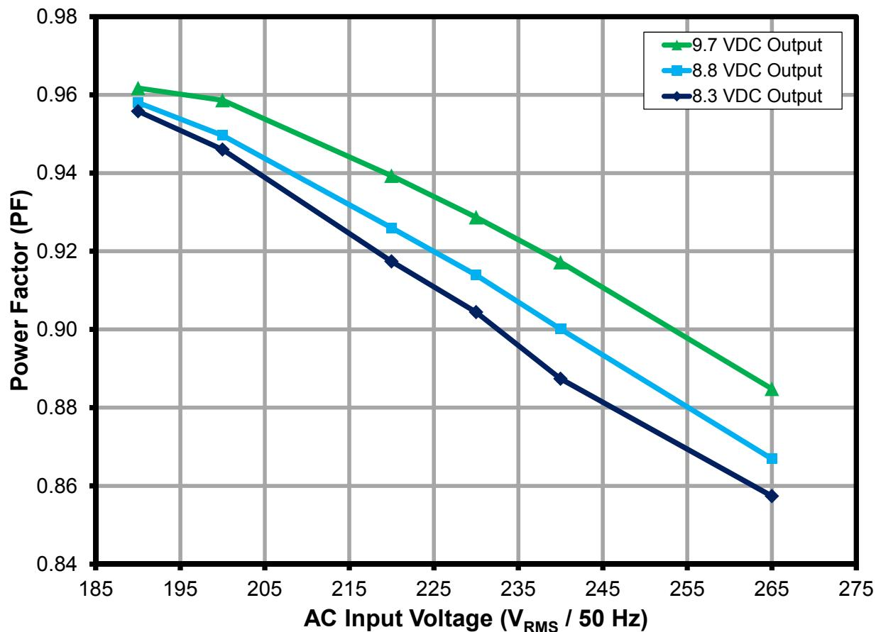
Figure 11 – High Power Factor within the Operating Range for 230 V LED.
