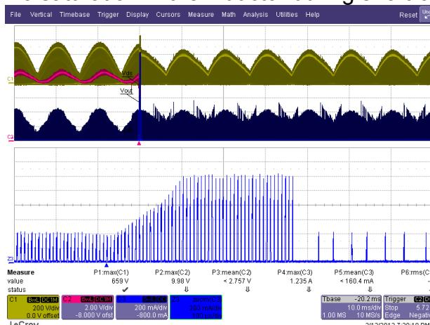
Figure 35 – 265 VAC / 50 Hz, Normal Operation then Output Short.
