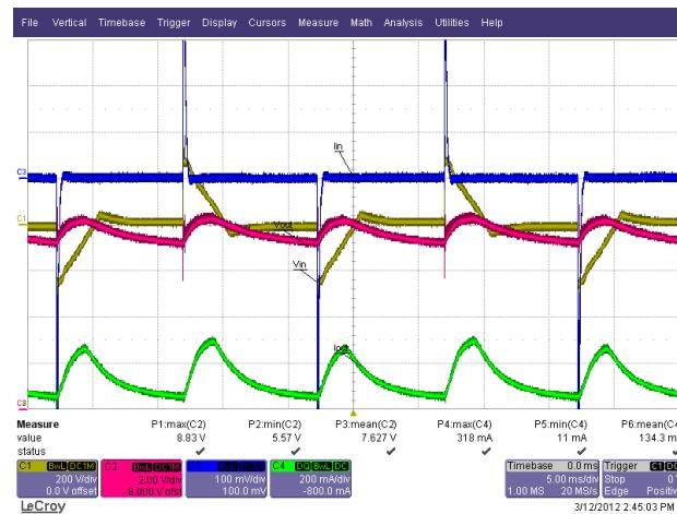
**Figure 48 – 230 VAC / 50 Hz, Sen Bo Lang Chinese Dimmer at Minimum TRIAC Conduction.**
