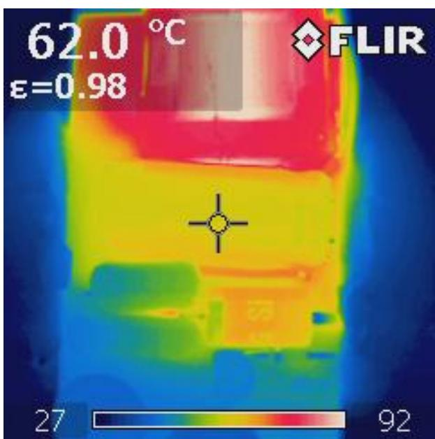
Figure 23 – C9 Output Capacitor.
