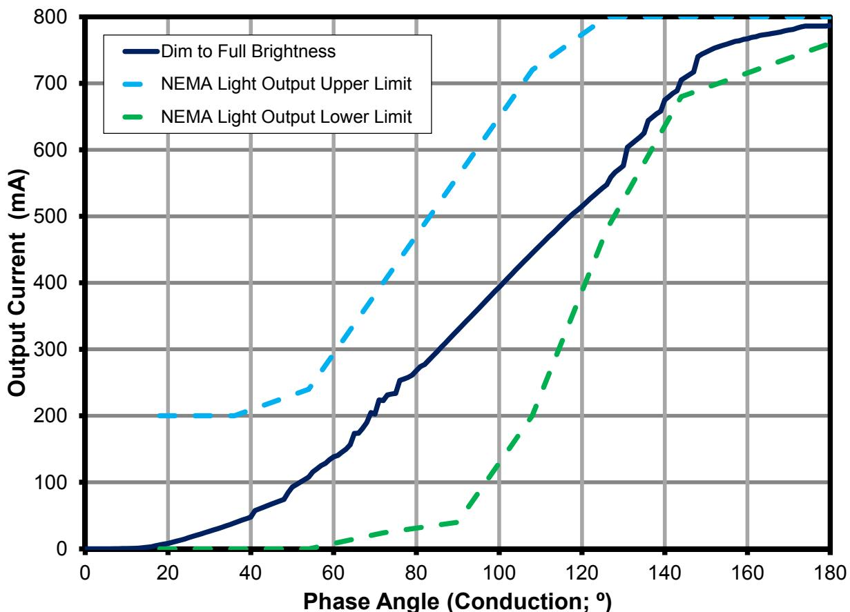
Figure 14 – Dimming Curve Characteristic from Full Dim to Full Brightness. Meets NEMA SSL 6-2010.
