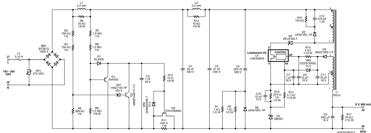
**Figure 2 – Schematic for 9 V / 800 mA PAR16 Replacement Lamp**
