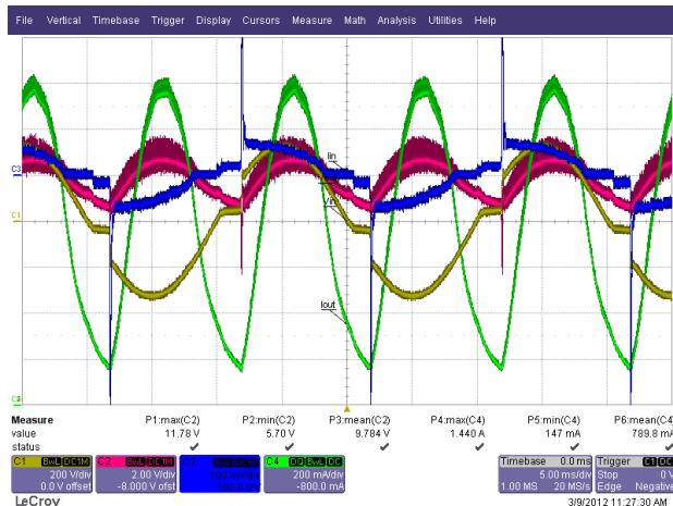
**Figure 49 – 230 VAC / 50 Hz, BUSCH2250 600 W German Dimmer at Full TRIAC Conduction.**
