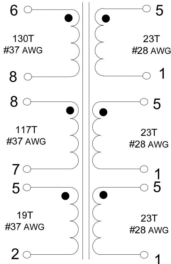
**Figure 7 – Transformer Electrical Diagram.**
