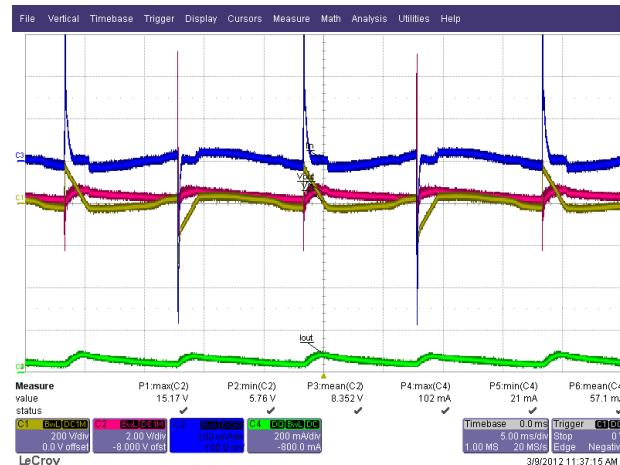
**Figure 50 – 230 VAC / 50 Hz, BUSCH2250 600 W German Dimmer at Minimum TRIAC Conduction.**
