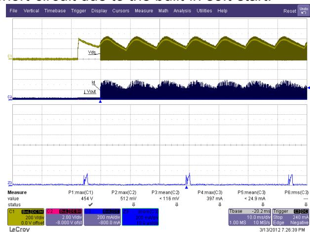
Figure 40 – 265 VAC / 50 Hz, Output Shorted.
