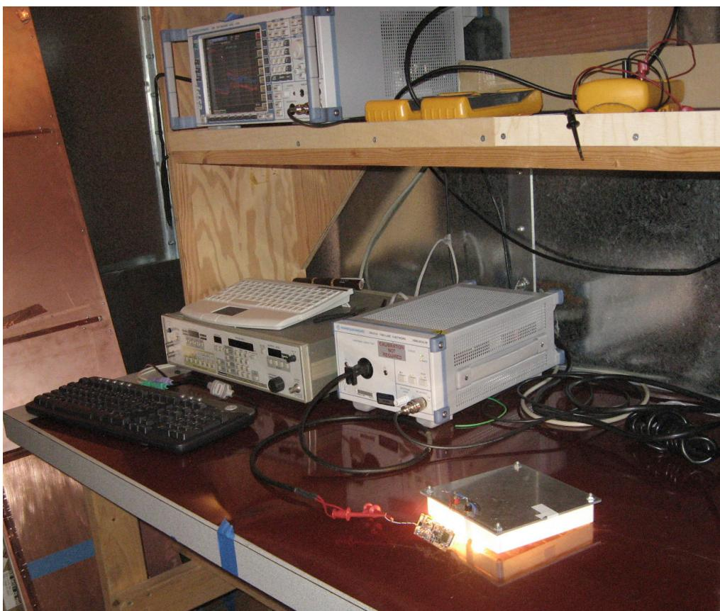
Figure 59 – Conducted Emissions Measurement Set-up.
