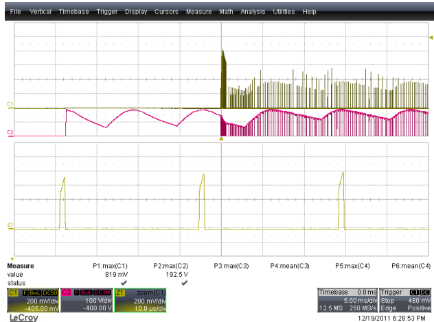
Figure 27 – 132 VAC / 60 Hz, 48 V LED String.
