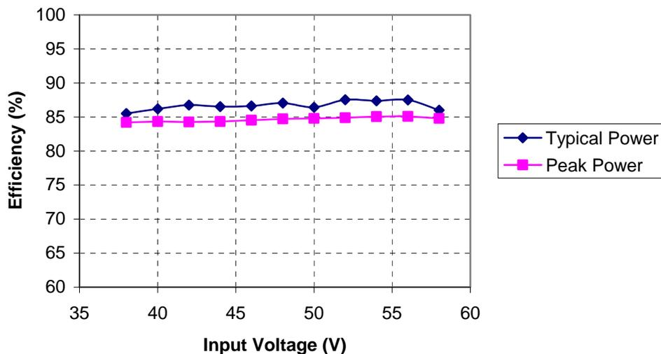
Figure 9 - Conversion Efficiency Variation with Input Voltage
