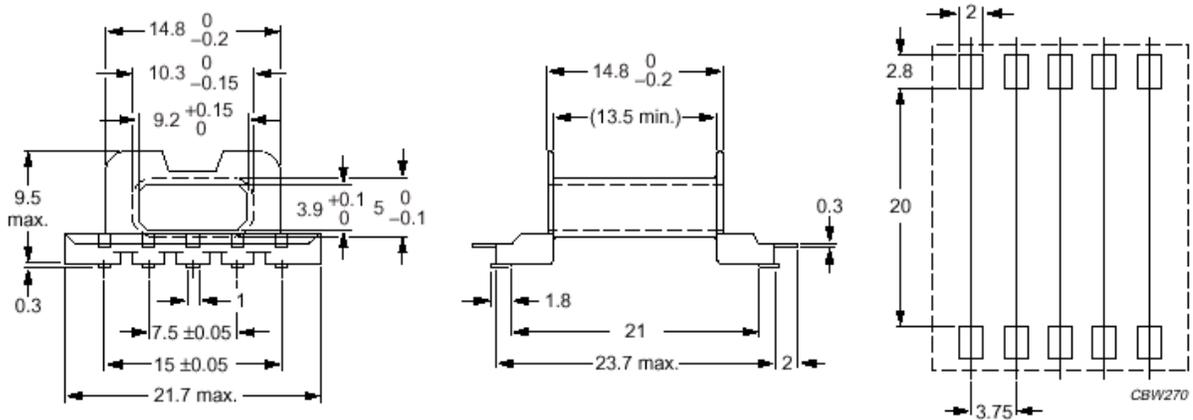
Figure 5 - 10 pin surface mount EFD20 bobbin
