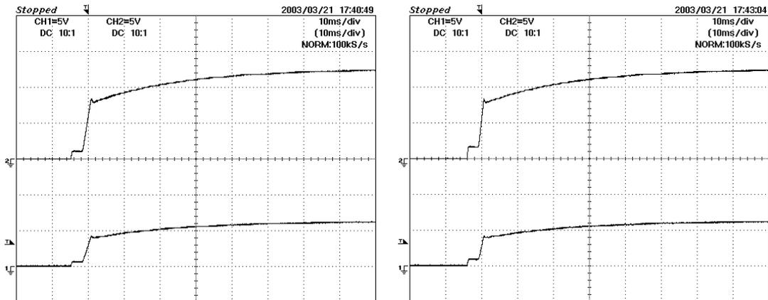
Figure 18 - 6V5 (Lower at 5V/div) and 12V5 (Upper 5V/div). Left hand graph is 38V input and right hand graph is 58V input
