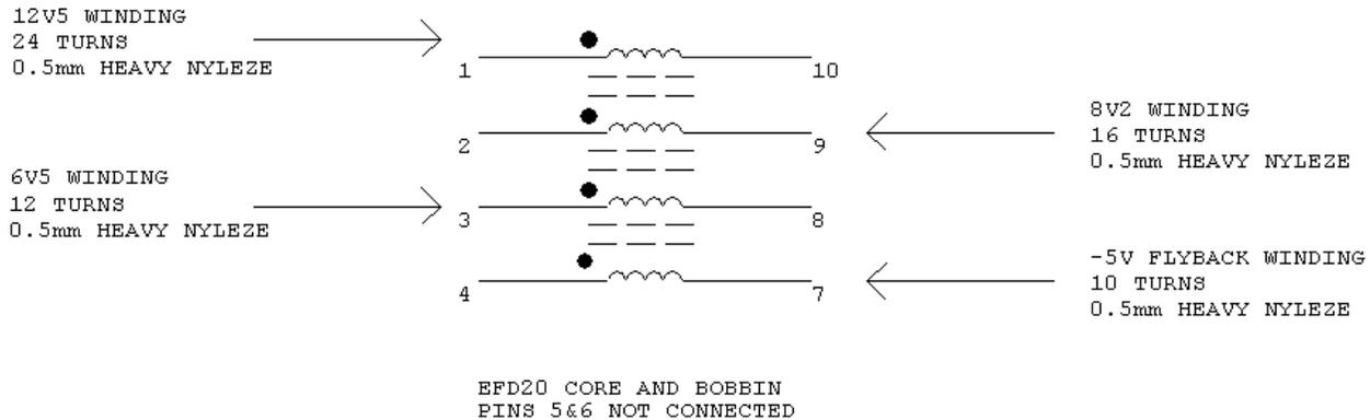
Figure 7 - Coupled Inductor Electrical Diagram
