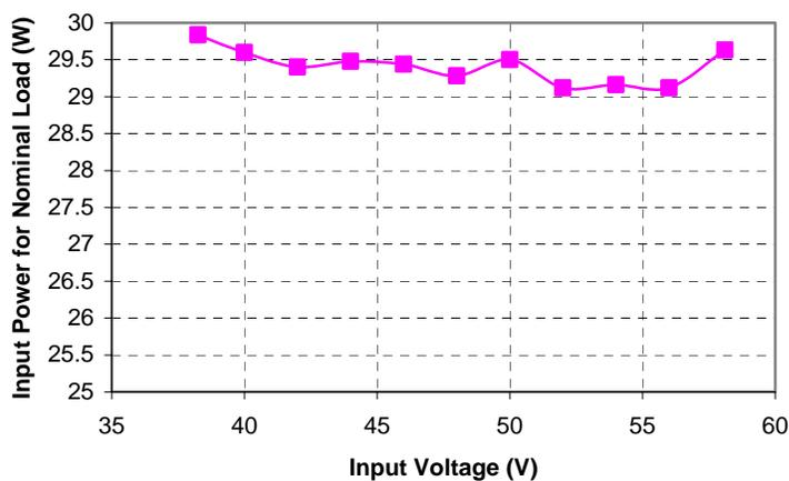
Figure 10 - Input Power at Nominal Load
