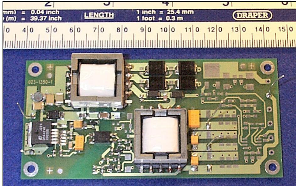
Figure 1 - Prototype DC/DC Converter (Scale in cm)
