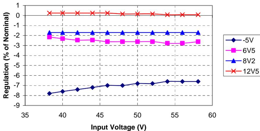
Figure 12 - Line Regulation under Nominal Load
