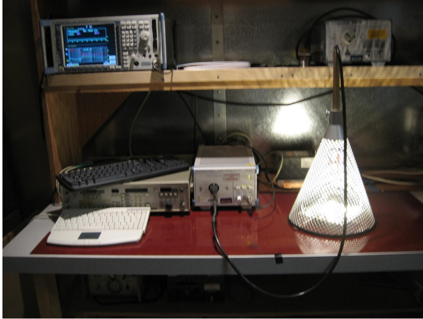
Figure 55 – EMI Test Set-up With the Unit and LED Load Placed Inside the Cone.
