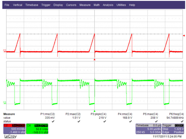
Figure 42 – 135 VAC, 60 Hz. Upper: I_{DRAIN} , 500 mA / div. Lower: V_{DRAIN} , 50 V, 5 μs / div.
