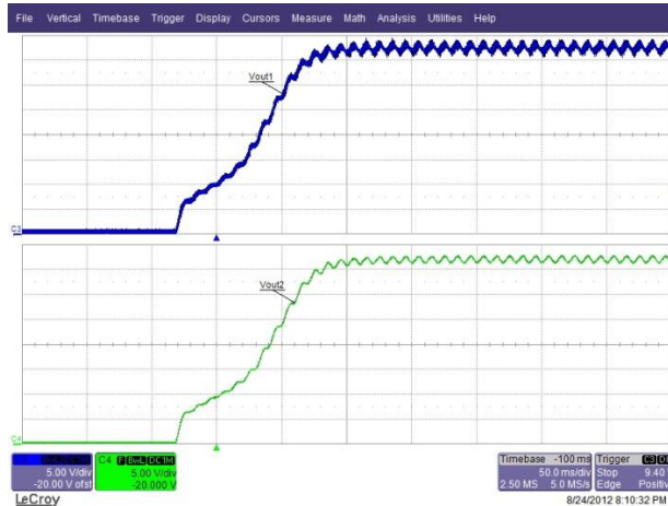
Figure 28 – 277 VAC 50 Hz, Power-down. Upper: V_{OUT-LED1} , 5 V / div. Lower: V_{OUT-LED2} , 5 V / div., 50ms / div.
