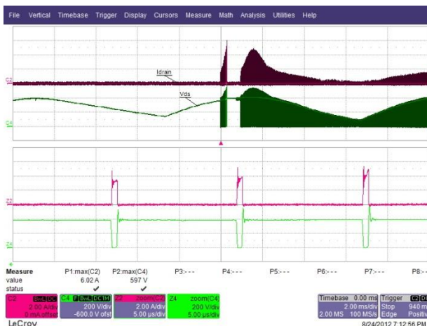
Figure 22 – 277 VAC 50 Hz., Full Load Start-up. Upper: I_{DRAIN} , 2 A / div. Lower: V_{DRAIN} , 200 V, 2 ms / div.
