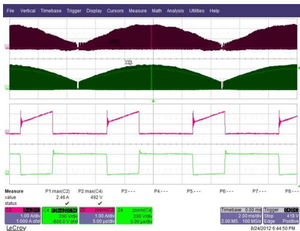
Figure 19 – 184 VAC 50 Hz, Full Load. Upper: I_{DRAIN} , 1 A / div. Lower: V_{DRAIN} , 200 V, 2 ms / div.
