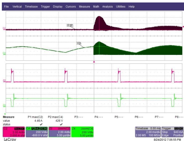
Figure 21 – 184 VAC 50 Hz., Full Load Start-up. Upper: I_{DRAIN} , 2 A / div. Lower: V_{DRAIN} , 200 V, 2 ms / div.
