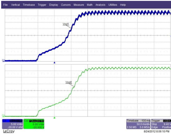
Figure 27 – 184 VAC 50 Hz, Power-up. Upper: V_{OUT-LED1} , 5 V / div. Lower: V_{OUT-LED2} , 5 V / div., 50ms / div.
