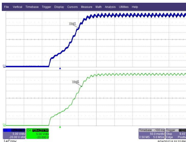
Figure 28 – 277 VAC 50 Hz, Power-down. Upper: V_{OUT-LED1} , 5 V / div. Lower: V_{OUT-LED2} , 5 V / div., 50ms / div.
