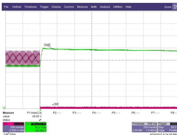
Figure 30 – 277 VAC 50 Hz, Output 2 Open. Upper: V_{OUT-LED1} , 10 V / div. Lower: I_{OUT-LED1} , 500 mA, 200 ms / div.
