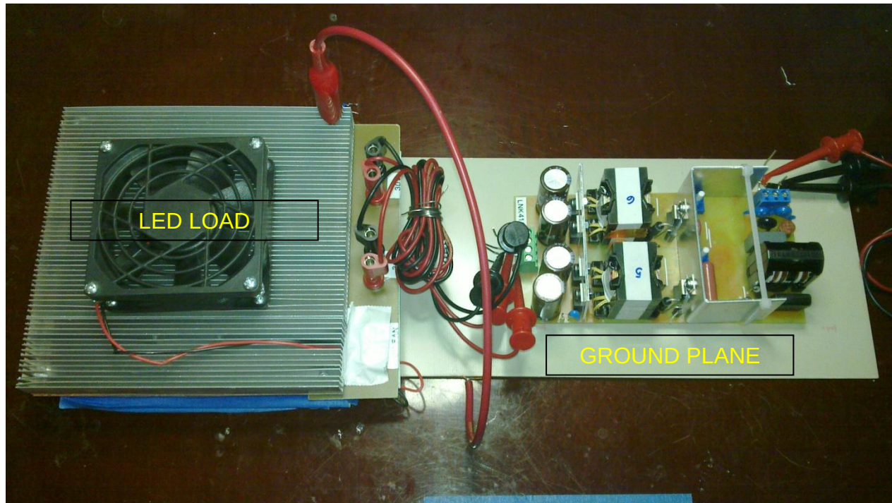
Figure 32 – EMI Measurement Set-up.
