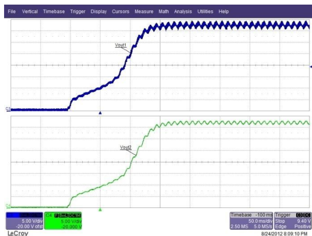
Figure 27 – 184 VAC 50 Hz, Power-up. Upper: V_{OUT-LED1} , 5 V / div. Lower: V_{OUT-LED2} , 5 V / div., 50ms / div.
