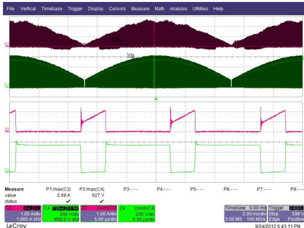
Figure 20 – 277 VAC 50 Hz, Full Load. Upper: I_{DRAIN} , 1 A / div. Lower: V_{DRAIN} , 200 V, 2 ms / div.
