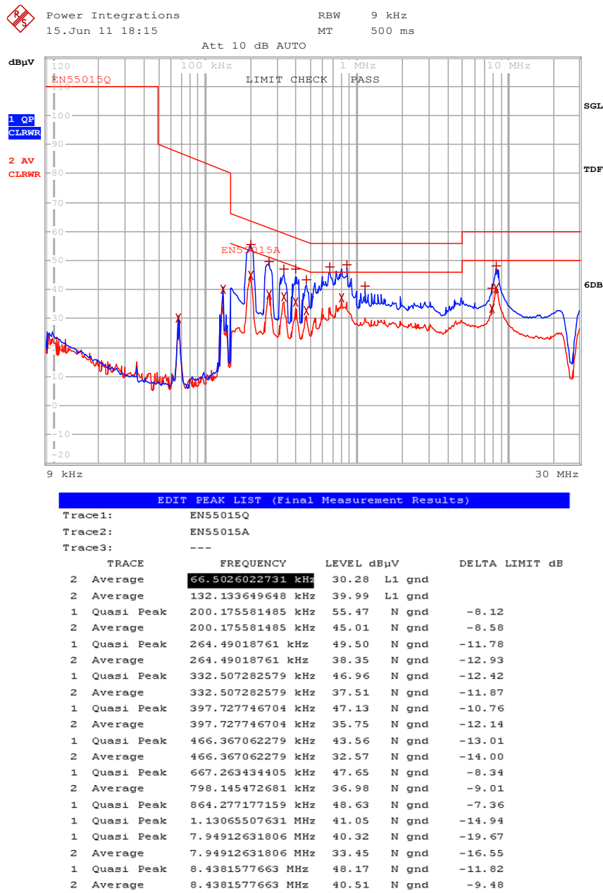
Figure 54 – Conducted EMI, 34 LED Load, 230 VAC, 60 Hz, EN55015B Limits.
