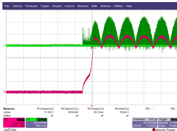
Figure 25 – 265 VAC, Full Load. Upper: I_{RIPPLE} , 0.2 A / div. Lower: V_{OUTPUT} , 5 V, 10 ms / div.
