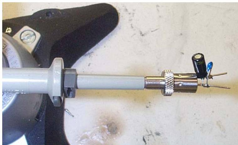
**Figure 20** – Oscilloscope Probe with Probe Master 4987BA BNC Adapter (Modified with Wires for Probe Ground for Ripple measurement and Two Parallel Decoupling Capacitors Added).
