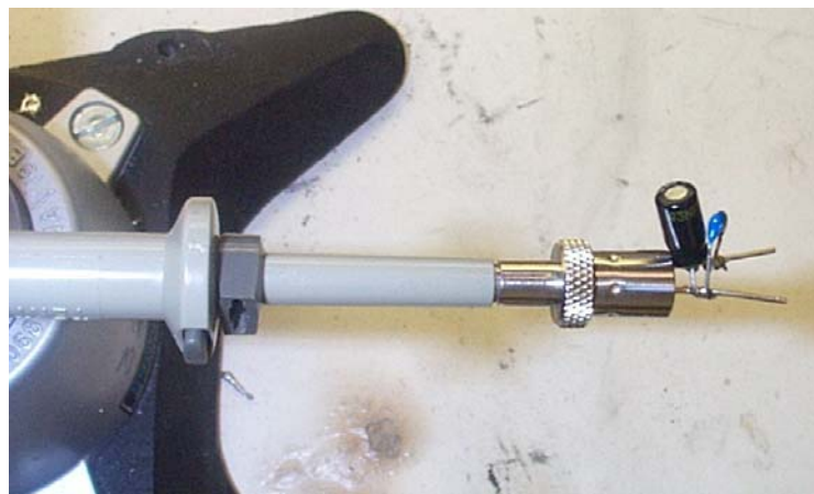
Figure 12 – Oscilloscope Probe with Probe Master 5125BA BNC Adapter (Modified with wires for probe ground for ripple measurement, and two parallel decoupling capacitors added)
