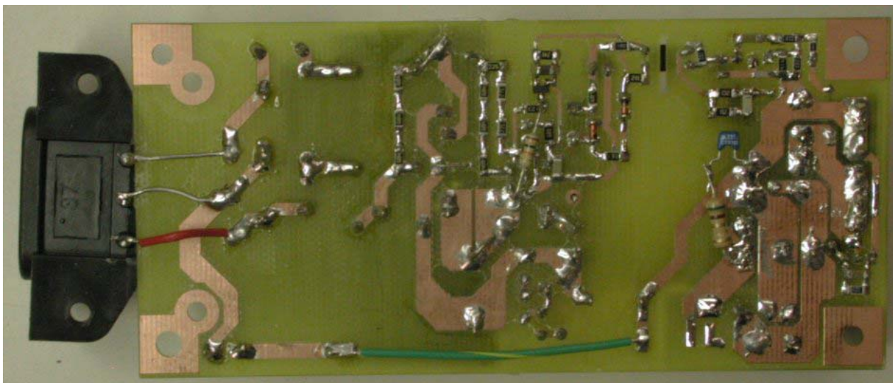
Figure 2 – LCD Monitor Prototype Power Supply – Bottom View
