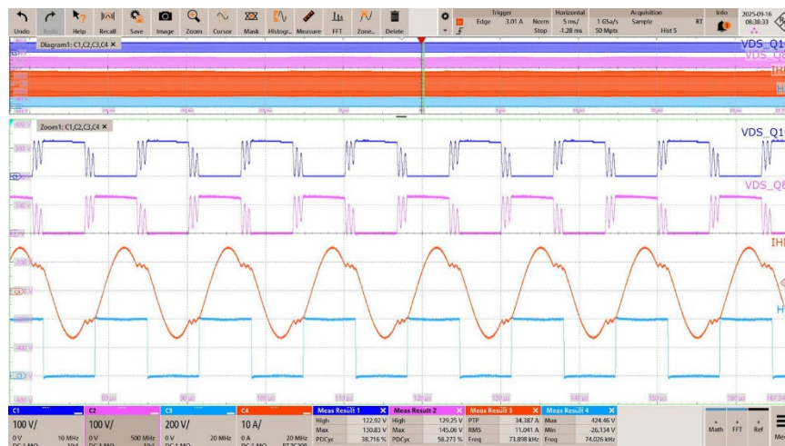
Figure 53 – Output Rectifier Peak Reverse Voltage at 60 V, 27.5 A.
